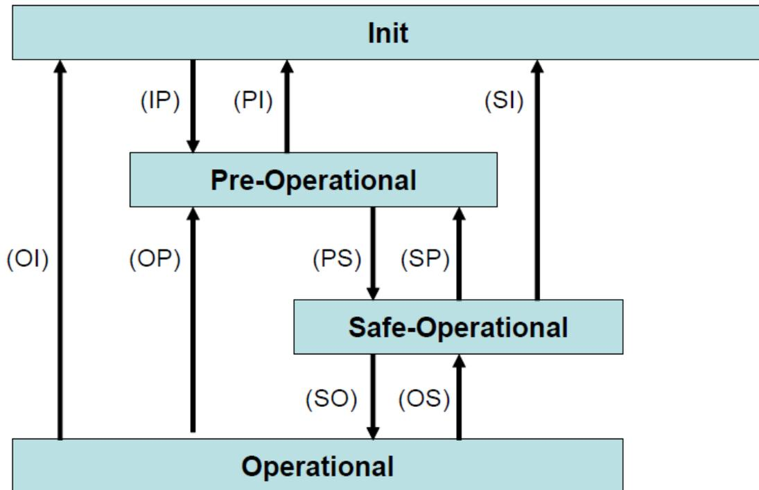
Figure 3: EtherCAT state machine
