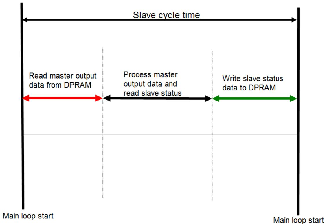
Figure 5: Slave processing sequence in Free-run mode
