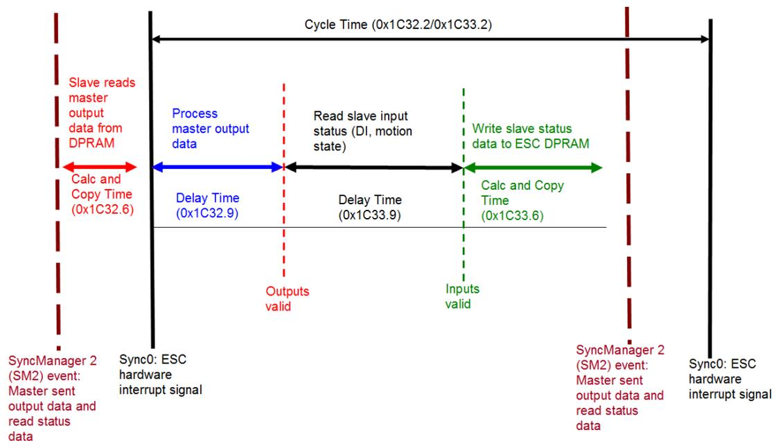
Figure 7: Internal slave processing sequence in DC mode
