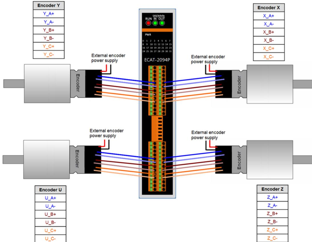
Figure 1: Encoder connection
