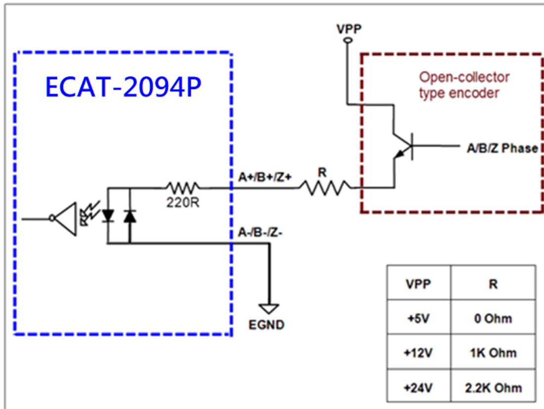
Figure 2: Open collector wiring diagram
