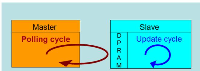
Figure 4: Master-slave cycle in Free Run mode
