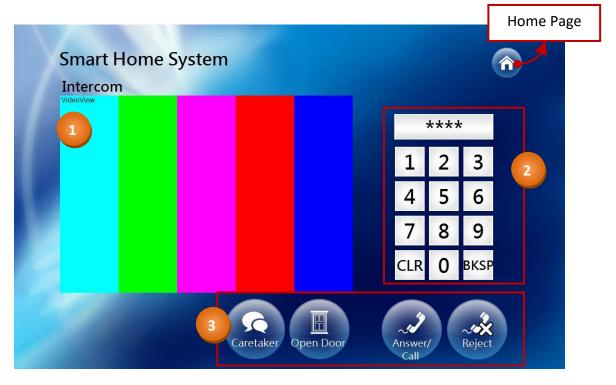
As illustrated above, the Intercom screen contains four sections. The following is an overview of the functionality of each of the sections that are displayed on the Intercom screen:
