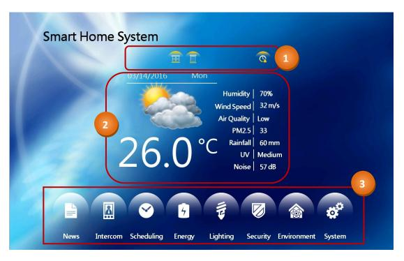
As illustrated above, the Home Screen contains three sections. The following is an overview of the functionality of each of the sections that are displayed on the Home Screen:
