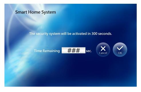
If an intruder is detected once the Smart Home system is armed, a countdown screen will be displayed for a fixed duration (60 seconds). The Smart Home system can be disarmed during the countdown period by tapping the **Disarm** button and entering the default password "1234" (see <u>Section 3.6 System</u>). If the Smart Home system is not disarmed within the fixed period, an alarm message will be sent to the building caretaker.
