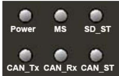
Figure 2-6 LED Assignment of CAN-Logger100
