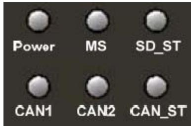
Figure 2-7 LED Assignment of CAN-Logger200
