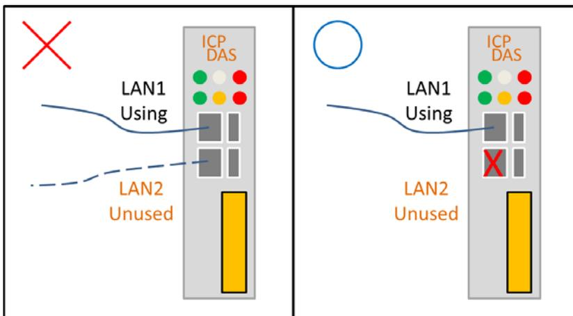
2. When both LAN1 and LAN2 are enabled, they **cannot** be set to the same network segment.
