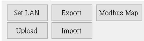
Set LAN: Configure the LAN1 and LAN2 IP Address of the DNP-211.
