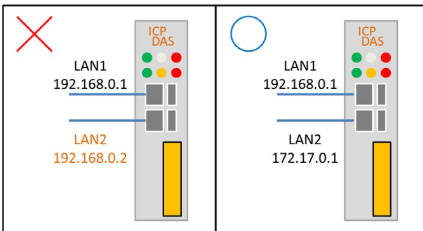
3. When both LAN1 and LAN2 are enabled, **they must be connected to two separate networks.**
