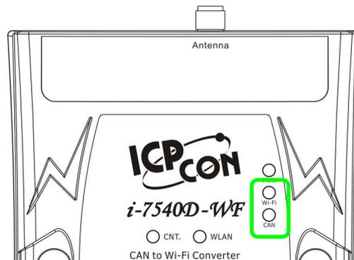
Figure 22: I-7540D-WF CAN and Wi-Fi Transmission LED
