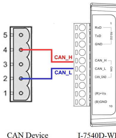
Figure 3: CAN bus Wire Connection
