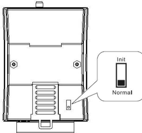
Figure 2: Operation mode Position of Dip-Switch
