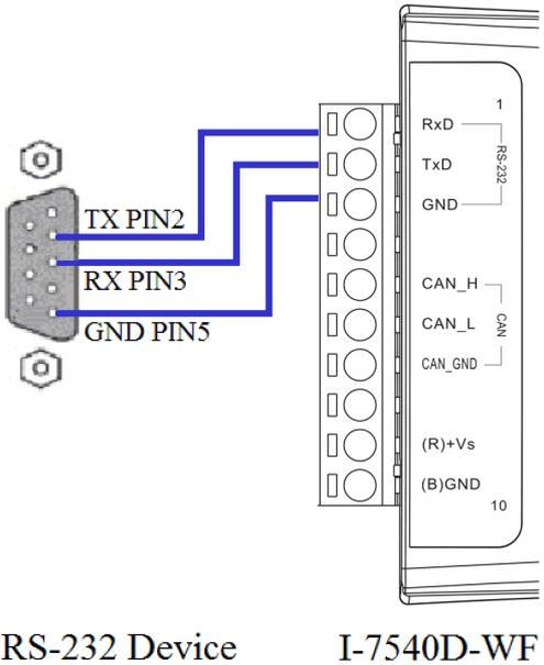
Figure 4: RS-232 Wire Connection
