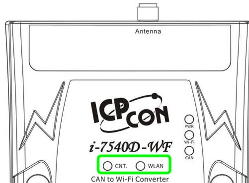
Figure 21: I-7540D-WF successful connection LED
