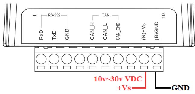
Figure 5: Power Wire Connection
