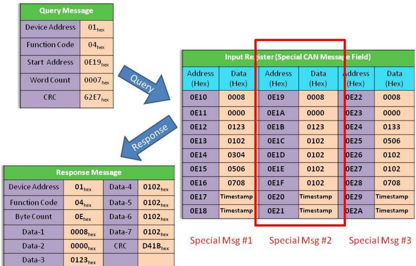
Figure 5-10: Use the Modbus RTU command to read specific CAN message.
