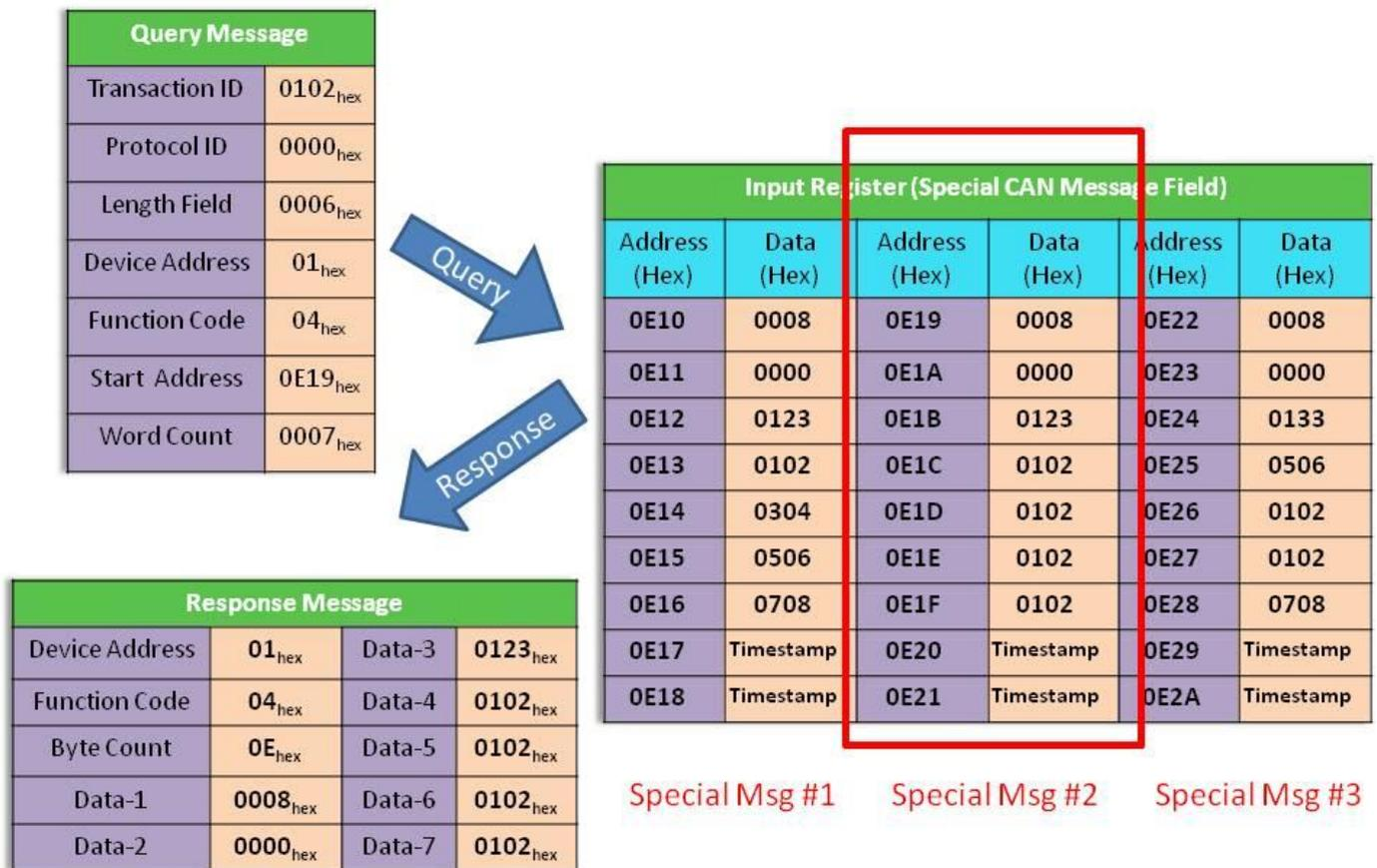
Figure 5-6: Use the Modbus TCP command to read specific CAN message.
