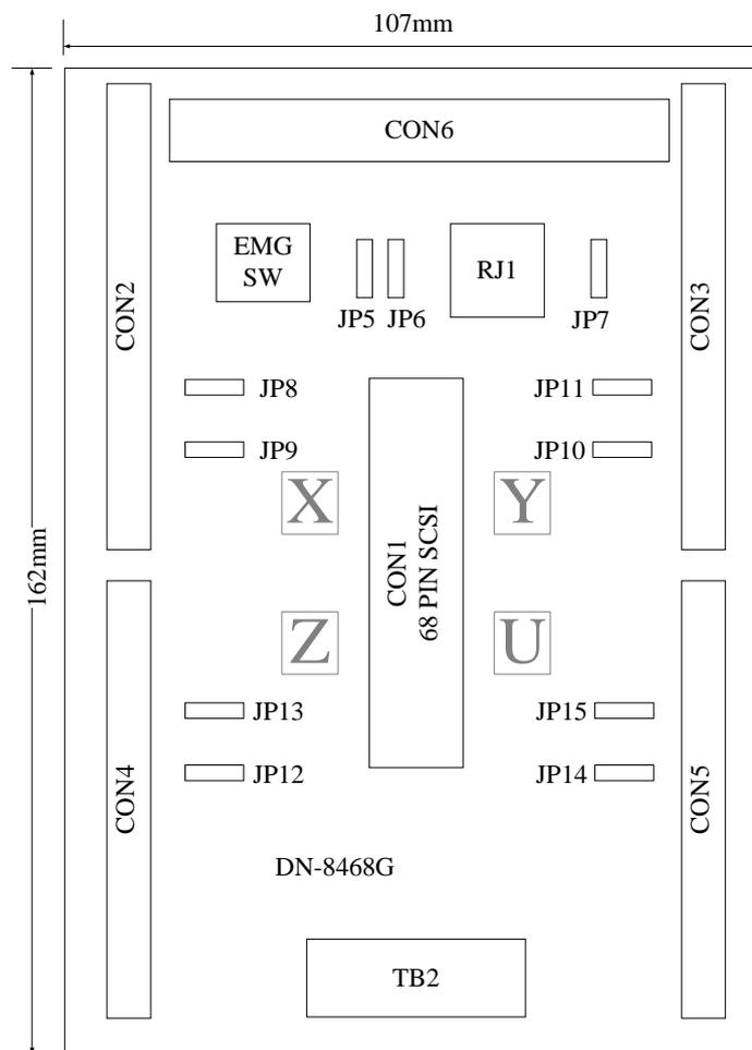
Fig. 1-1 Board layout for the DN-8468GB
