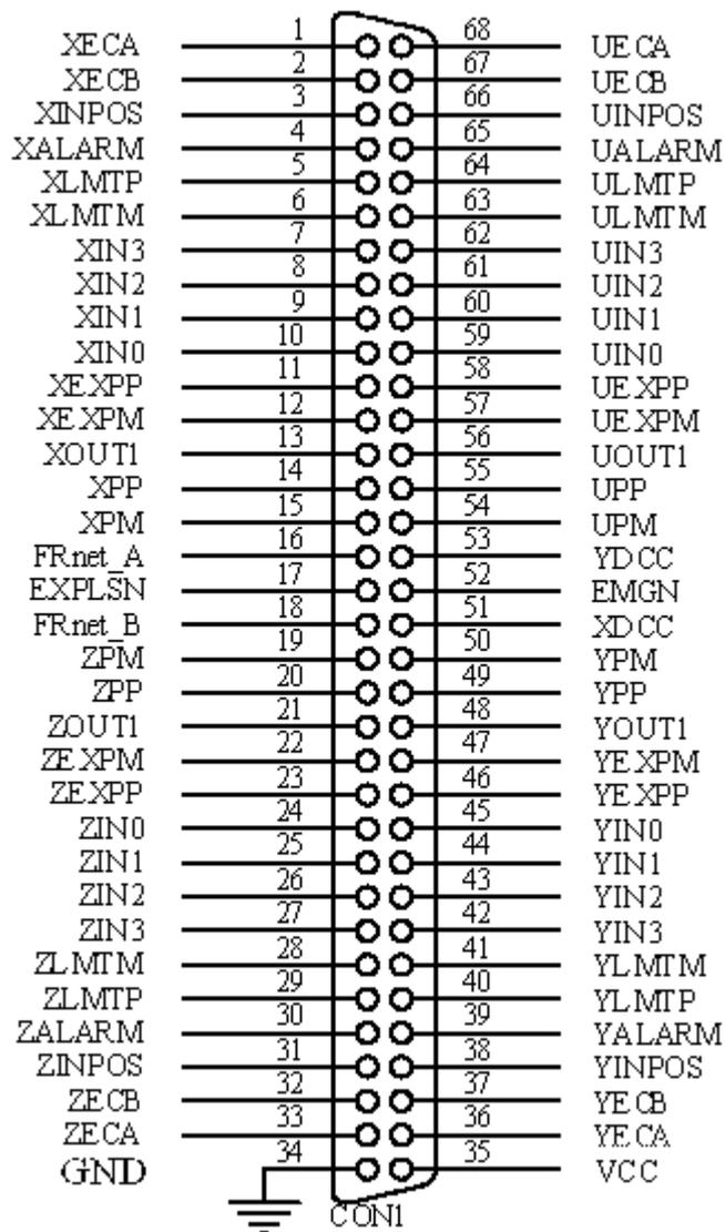
Fig. 1-2 I/O connector pin assignment for the CON1
