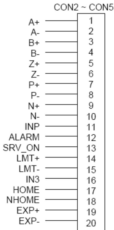
Fig. 1-3 Pin definition for CON2 ~ CON5
