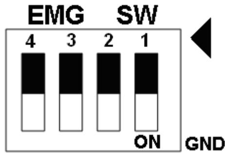
Fig. 1-9 EMG SW setting for user controlled signals.
