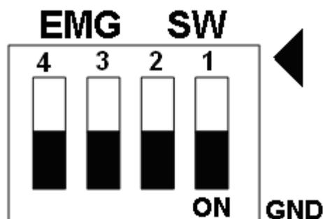
Fig. 1-8 EMG SW setting for normally GND (Default setting)
