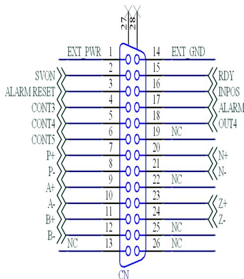
Fig 3-5 Pin definition for CN-X, CN-Y, CN-Z, CN-U
