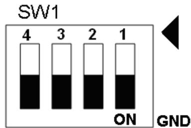
Fig. 3-13 SW1 setting for normally GND (Default setting)
