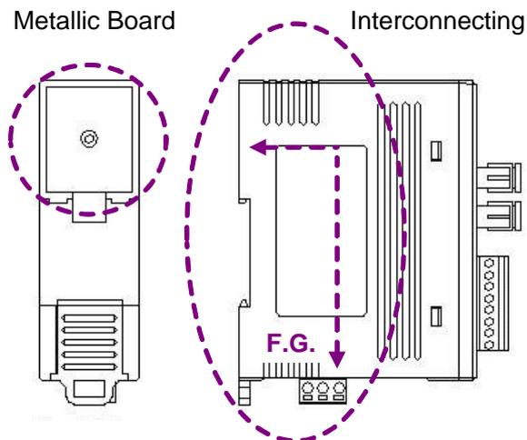
Figure 2-7 Metallic Board at Back of I-2532
