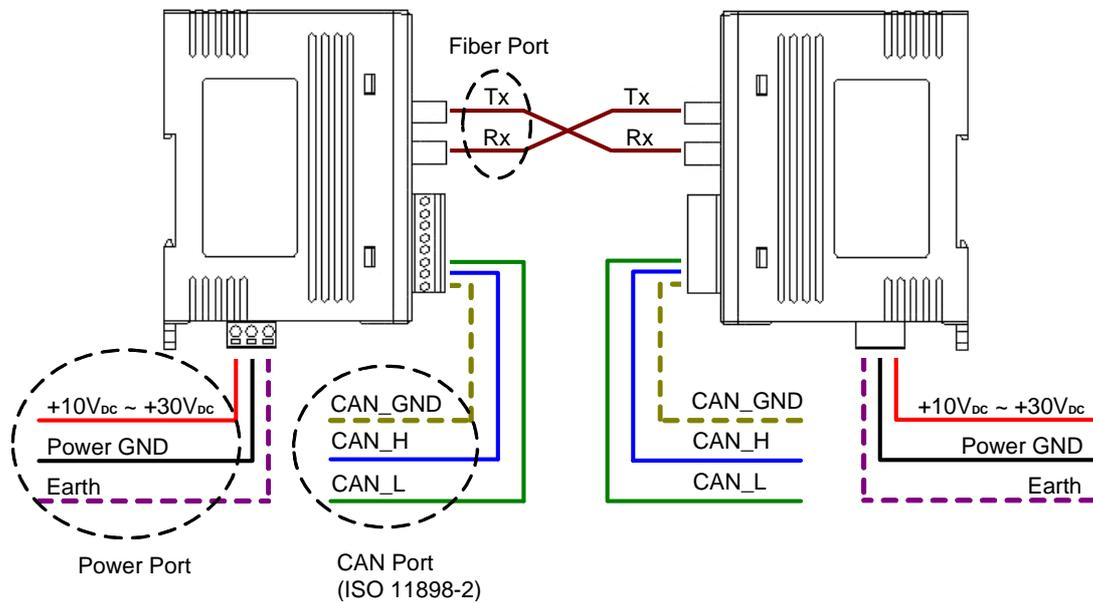
Figure 2-6 Wire Connection of I-2532
