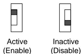
Figure 2-4 Adjustment of Terminal Resistance
