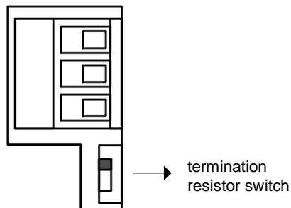
Figure 2-3 Location of Terminal Resistance Switch
