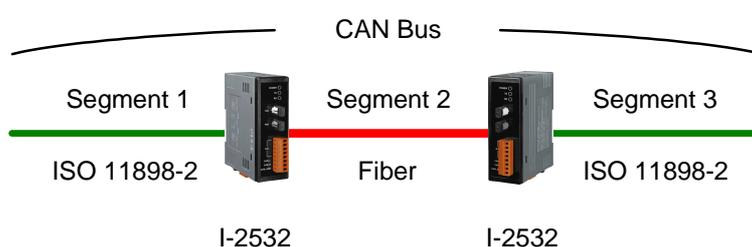
Figure 3-1 Segment in CAN bus system
