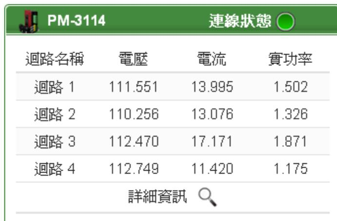
The screenshot shows a software interface for a PM-3114 device. At the top, there is a green header bar with the device name 'PM-3114' and a '連線狀態' (Connection Status) indicator, which is a green circle. Below the header is a table with four columns: '迴路名稱' (Circuit Name), '電壓' (Voltage), '電流' (Current), and '實功率' (Real Power). The table lists four circuits with their respective values. At the bottom of the table, there is a '詳細資訊' (Detailed Information) button with a magnifying glass icon.
