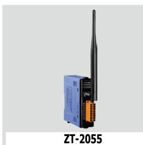
Wireless 8-channel Isolated Digital Input and 8-channel Isolated Digital Output Module
