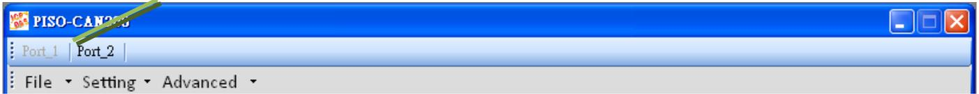
Users can switch the tag to change the activated virtual CAN port of the selected CAN devices for accessing the CAN network.
