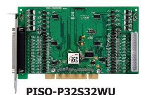
Universal PCI, 32-ch Optical Isolated DI and 32-ch Open Collector Isolated (Sink, NPN) DO Board
