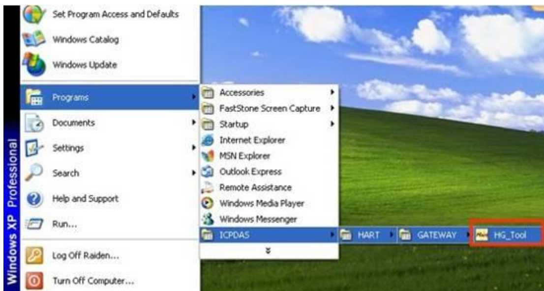
Figure 52: Run “HG_Tool” Utility
