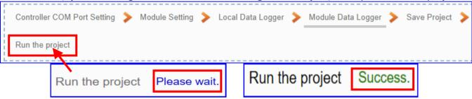
When the words "Please wait" disappears, the new words "Success" appears, that means the UA controller is running new project successfully. Then the Step Box will disappear automatically now, and back to the first screen view of the Web UI.
