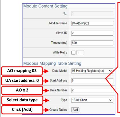
> Modbus Mapping Table Setting: Set module in the order of Data Model, Start Address and Data Number, then click "Add".
