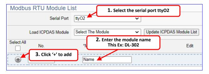
Add a module (as the picture, this example: **DL-302**), and then click the [Edit] of the module to enter the screen of "Module Content Setting".
