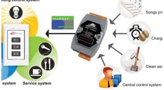
architecture, ISaGRAF PAC works as an agent controller for information exchange and for linking actions and communication between newly-added service and the original operations of the KTV system.
