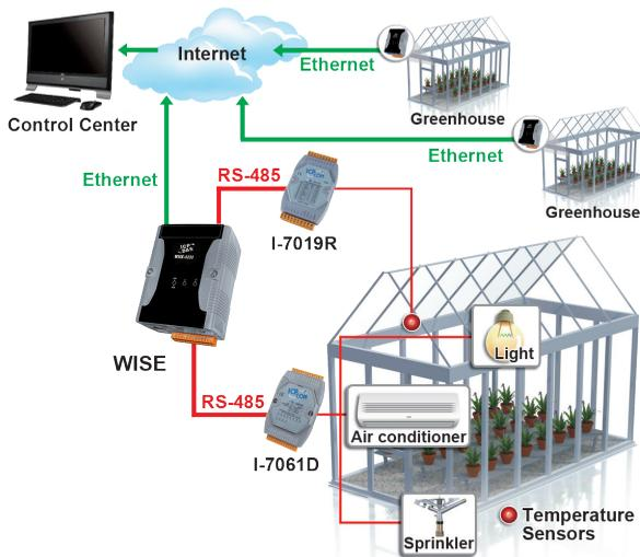
In addition to the Modbus TCP/RTU slave function that enables SCADA system to poll the I/O channel data of the WISE, now WISE provides “Active I/O sending” mechanism (Modbus TCP master, SNMP Trap and MQTT publish). Based on the “Active I/O sending”, WISE allows to send the
