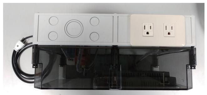
For power measurement, we use 110 to 220VAC power supply as a reference voltage, and clip the Current Transformer to the output circuit so it can measure the power data of the circuit.
