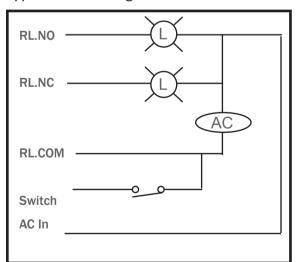
When the "Switch AC In" pin detects a change, the relay output status will change immediately without needing to pass through software control.
