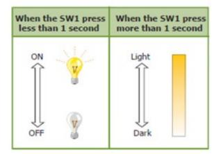
The LC-221 analog output is used to control dimmer switches connected to light sources. The "Switch AC In" pin can be connected to a control switch, which can be used manipulate fluorescent lights depending on the length of time the switch is pressed, for example, pressing for <1 sec. will switch the lights on or off, whereas pressing for >1
