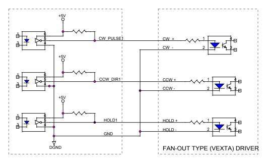
Fig.(11) fan-out type driver (VEXTA's motor driver)
