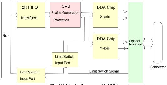
Fig.(1) block diagram of I-8091 card
