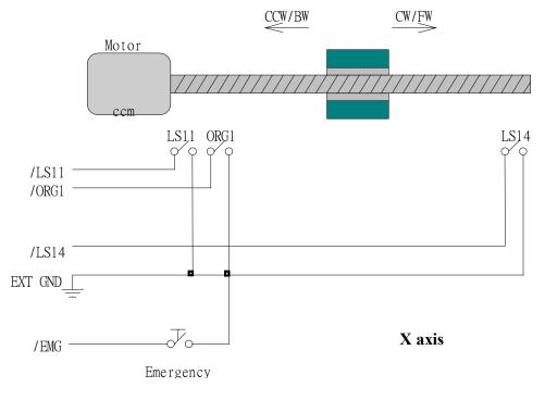
Fig.(5) Limit switch configuration of X axis
