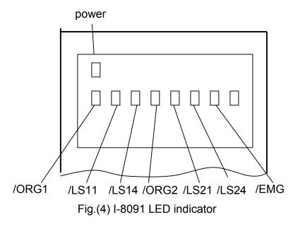
/ORG1: X-axis's original limit switch for machine home position.
