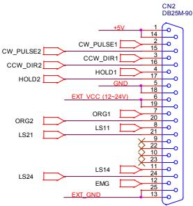
Fig.(8) CN2 connector of I-8091
