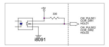
Fig.(9) internal circuit of pulse output pin
