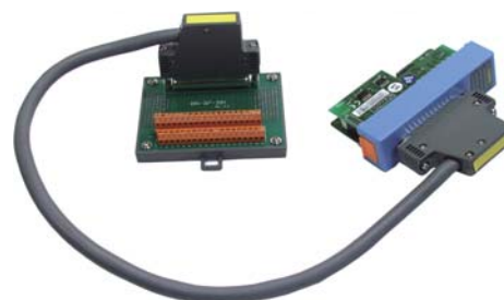
i-8040/ 41/ 42 and i-87040W/ 41W with DN-37-381-A
