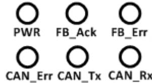
Figure 2-5 LED Assignment of I-2533CS
