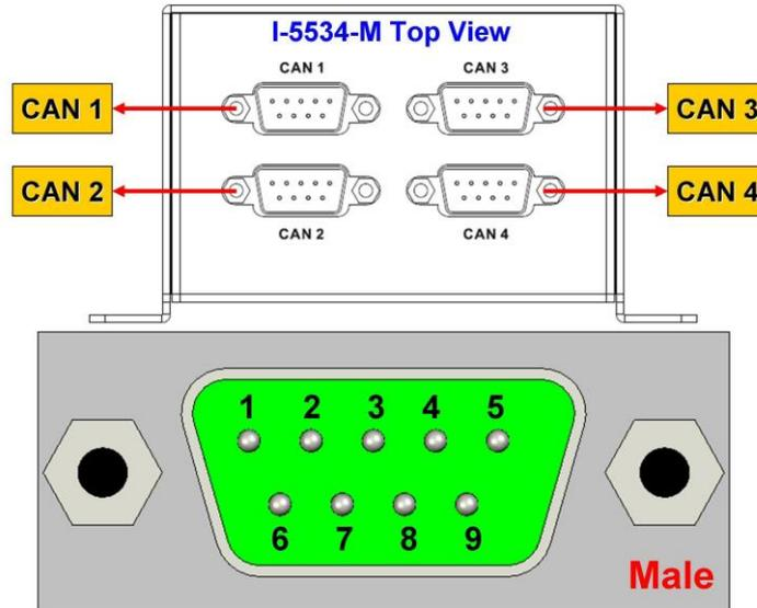
Figure 2-3 CAN bus pins of the I-5534-M
