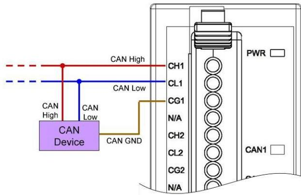
Figure 2-18 CAN bus wire connection with the I-2534 module
