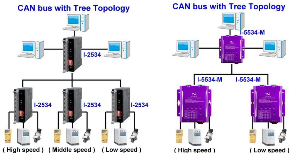
Figure 3-2 Tree topology with the I-2534 and I-5534-M
