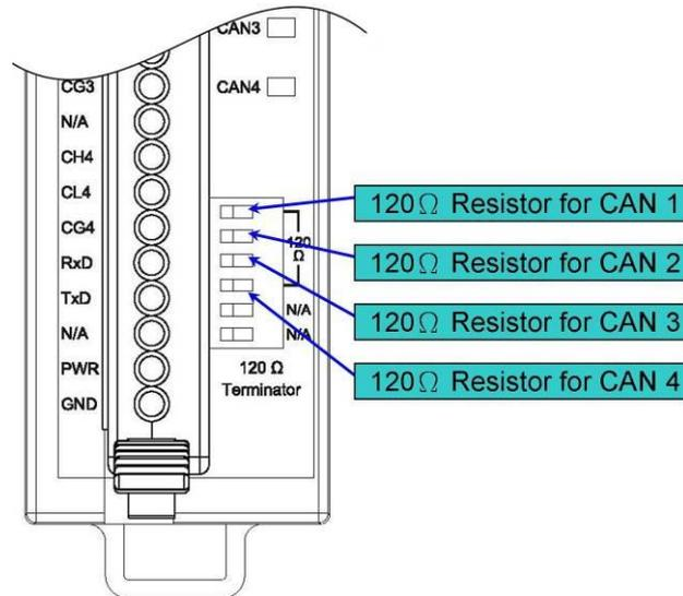
Figure 2-8 120Ω terminal resistors of the I-2534
