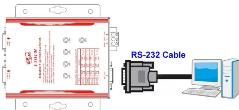
Figure 3-6 RS-232 wire connection of the I-5534-M
