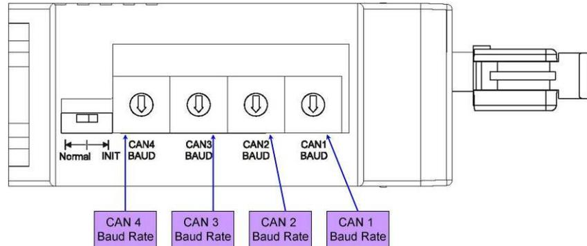
Figure 2-14 CAN baud rate configuration
