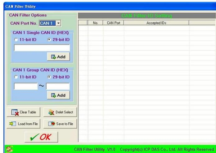
Figure 3-12 CAN filter configuration dialog
