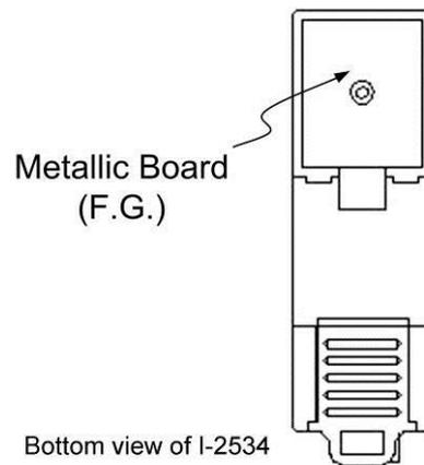
Figure 2-19 Metallic Board at Back of the I-2534
