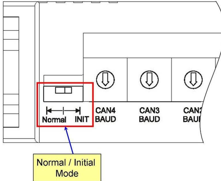
Figure 2-16 Operation Mode of the I-2534 module
