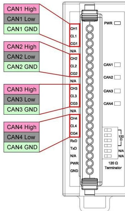
Figure 2-2 CAN bus pins of the I-2534
