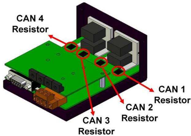
Figure 2-9 120Ω terminal resistors of the I-5534-M
