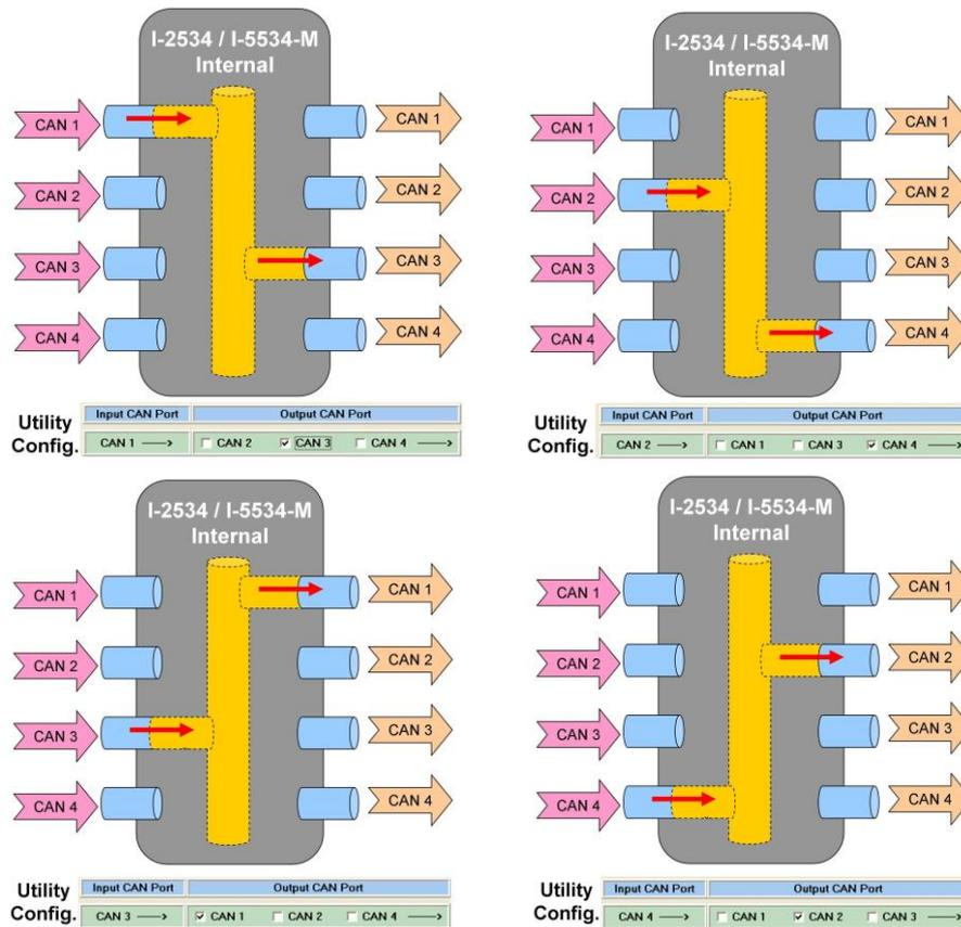
Furthermore, how to share the CAN bus into four or more CAN networks? The users can use three I-2534 or I-5534-M modules to achieve this requirement. Here shows the figure.
