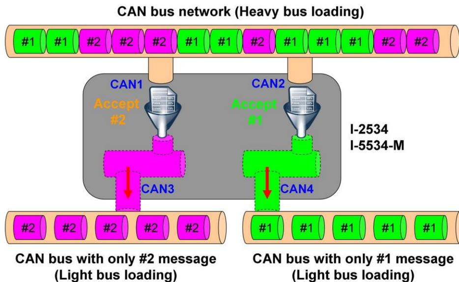
4. The route path needs to be configured as CAN1 <-> CAN 3, CAN2 <-> CAN 4.
