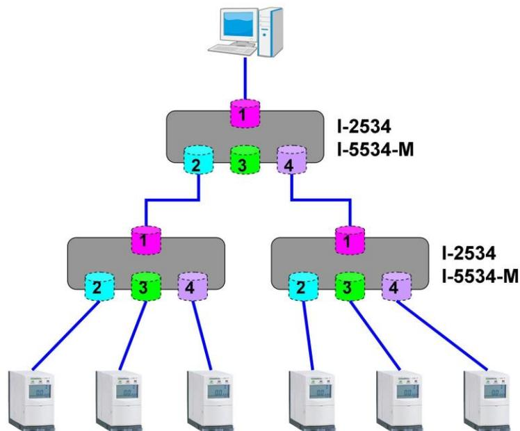
2. Configure the route path to make the response message only send to the PC side. All of the I-2534s or I-5534-Ms can be configured as follows.
