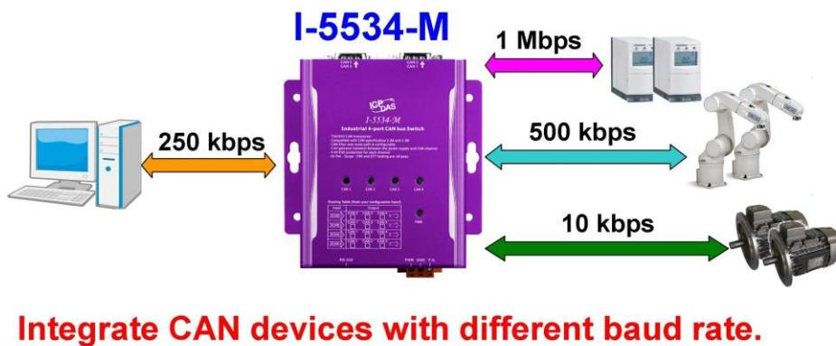
Figure1-2: Application to integrate the devices with the different baud rates.
