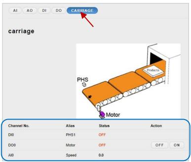
On the **Carriage** page, you can click the control button of the motor to set it as ON. For testing, when the AI value is "5", the value will be converted to a conveyor speed of  $5 \times 0.25 = 1.25$  (m/s)
