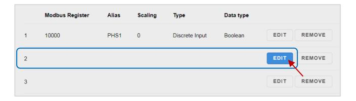
Step 7: Add a DO that is to be used to write the "Motor" output to turn the conveyor motor on and off
