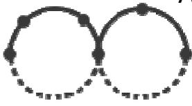
As a ring network is a small group of switches by geography, functionalities, or subsystem, 2 or more rings could be coupled together to form a whole picture of industrial network for an integrated system.
