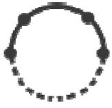
A ring topology ensures the network having one more chance to keep connection alive when any connection between 2 switches (nodes) has been broken inside the ring.
