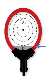
The diagram below shows the variation of accuracy throughout the coil. The variation is greatest when the current is positioned near the junction of the connecting cable and the coil, where there is some discontinuity, and the error here can be typically 5%. Since in most applications the current is distributed throughout a significant part of the area contained by the coil loop the reading will be very close to the calibration value.
