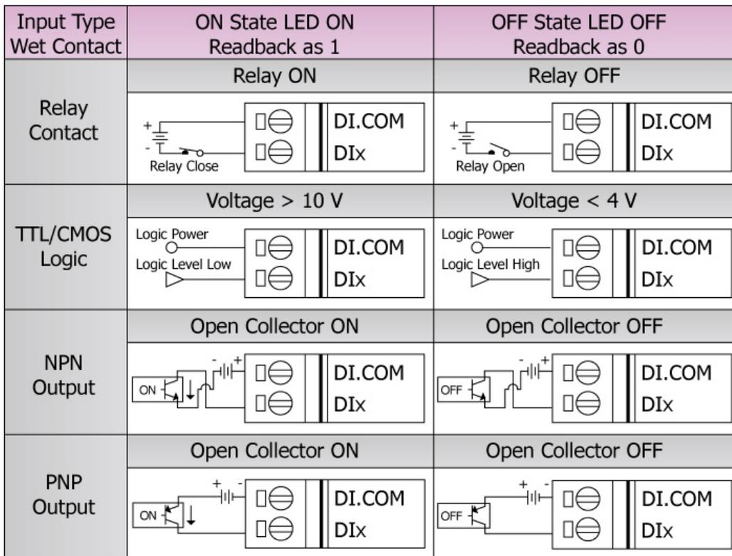
Figure 2-14: DI Wet contact wire connection of WF-2055
