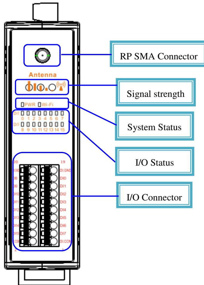
Figure 2-1: Front Panel of the WF-2000(DIO)
