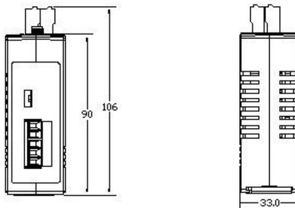
Figure 2-8: Top / Bottom dimension of the WF-2000
