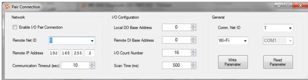
Figure 3-5: Pair connection configuration screen
