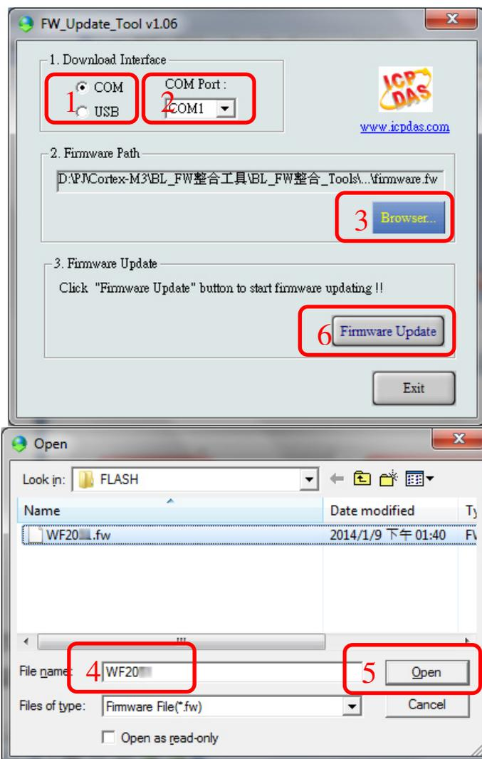
Figure 2-23: WF-2000 firmware update process
