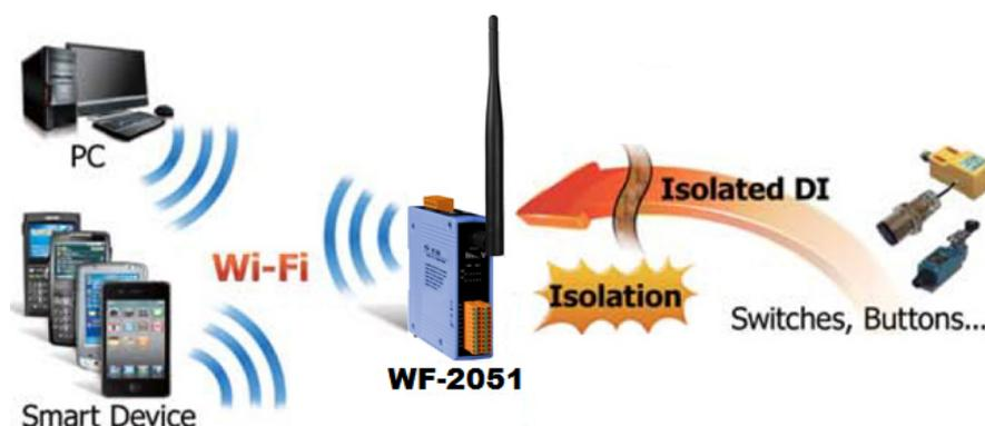
Figure 4-1: WF-2051 + Laptop application architecture
