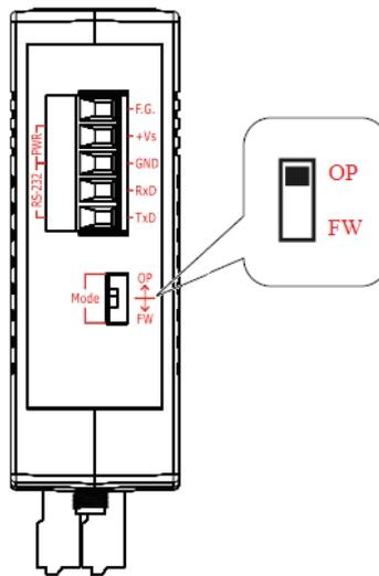
Figure 2-24: OP Position of Dip-Switch
