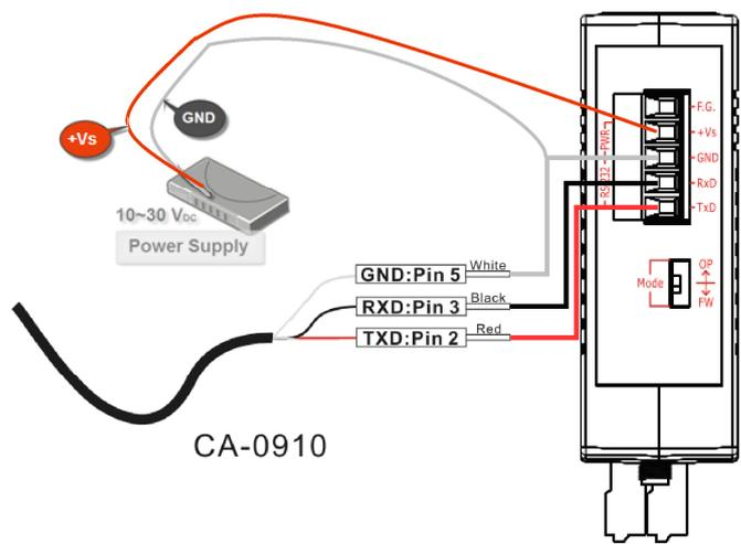
Figure 2-9: Power and Serial port wire connection
