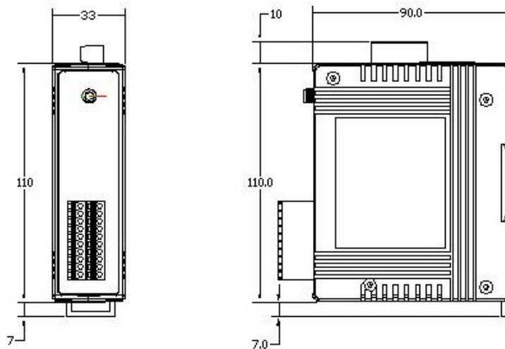
Figure 2-7: Front / Left Side dimension of the WF-2000
