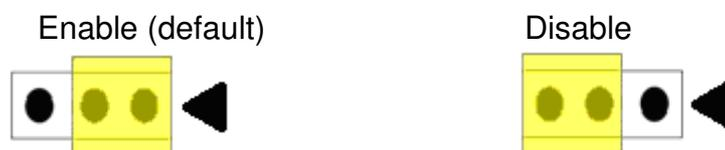
Figure 2-19: Watchdog timer Jumper Position
