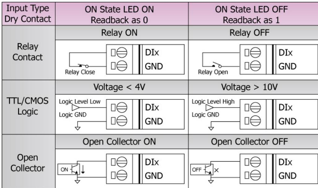
Figure 2-13: DI Dry contact wire connection of WF-2055
