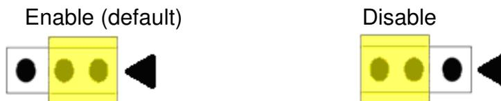
Figure 2-19: Watchdog timer Jumper Position
