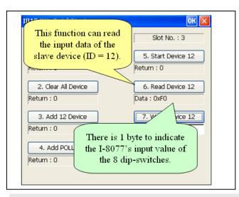
12. In this step, users can edit the output data. And send the data to the output channel of the slave device (ID = 12) by pressing "Write Device 12" button to send the output data to the output channel of the slave device (ID = 12). At the same time, the D/O LED on I-8077 will show the same value.
