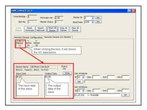
10. Press "Write" button to send the output data to the slave device.
