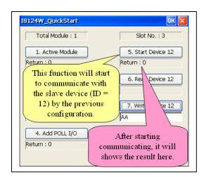
11. In this step, users can press the "Read Device 12" button to read the input data of the slave device (ID = 12). The input data is from the I-8077's 8 dip-switches. After changing the dip-switches, users can press the button again to refresh the LED status.
