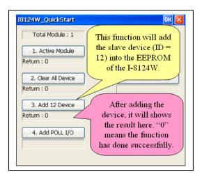
9. In this step, the user can press the "Add POLL I/O" button to add the Poll connection information of the slave device (ID = 12) into the EEPROM of the I-8124W.
