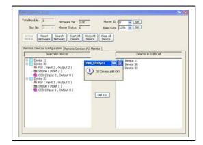
7. Press "Start all Device" button to communicate with all slave devices.
