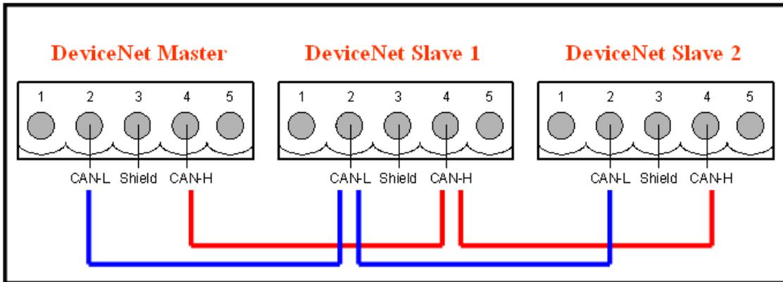
The following wire connection is **wrong** which is shown as follows.
