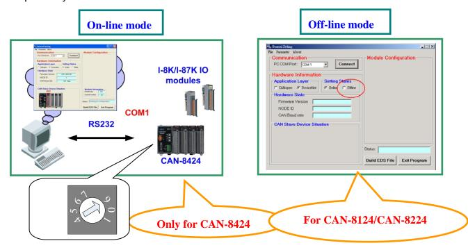
Note: In the on-line mode, users can define the needed assembly instance or default assembly instance, and set the IO connection path. But in off-line mode, we provide the default assembly instance for the CAN-8124/CAN-8224. The IO connection path must be set via an explicit connection.
