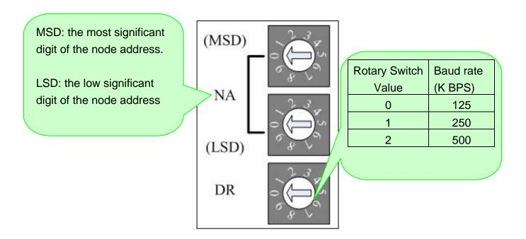
Note: If users set the illegal values of the rotary switch, the MOD led will flash when the system is powered up. If this condition occurs, users must configure the legal values of the switches and reset the device, and then the device should work normally.
