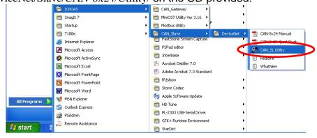
**Step 2:** There are 2 modes in the CAN Slave Utility. One mode is off-line and it allows users to create EDS files off-line for the CAN-8x24. Another mode is on-line mode. Before using the CAN Slave utility in the On-line mode with the CAN-8424, please make sure that you have connected the COM1 port to the CAN-8424 with the available COM port on your PC.
