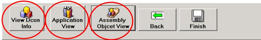
**Step 11:** The last step is to press the “Finish” button to create the EDS file and store these information into the i-7241D’s EEPROM. You can find the EDS file “DNS\_DCONx.eds” in the path of CAN\_GW.exe.
