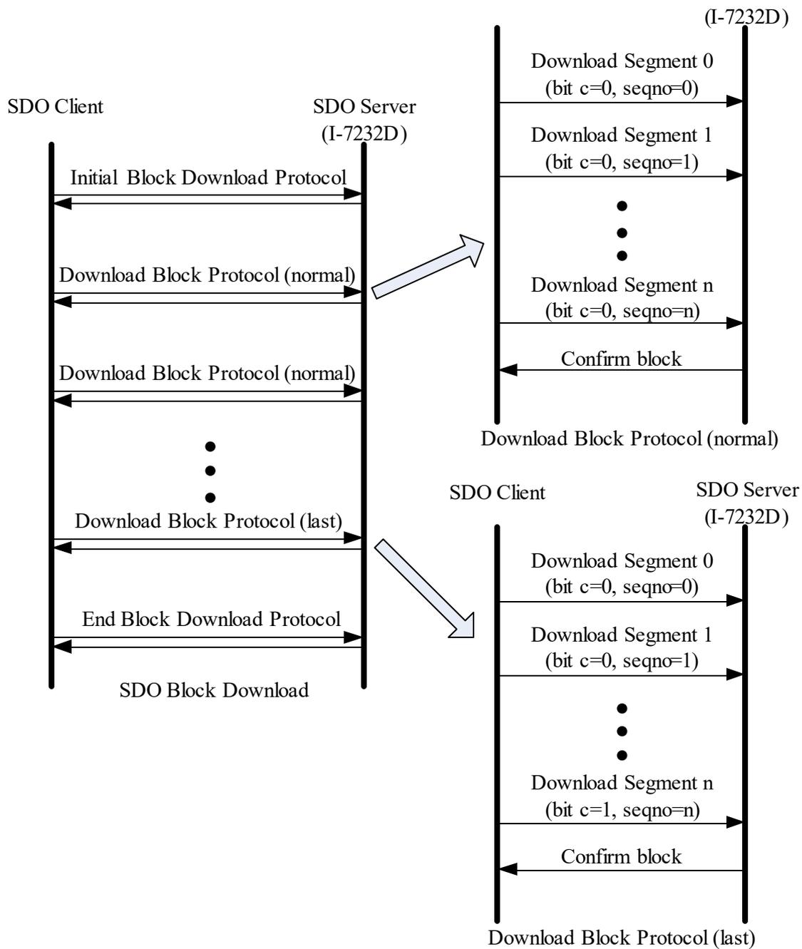
Step 1. In order to inform the I-7232D that the value of the object entry with index 0x1400 and sub-index 02 will be modified by using the SDO Block Download method, the Initiate SDO Block Download protocol is implemented.
