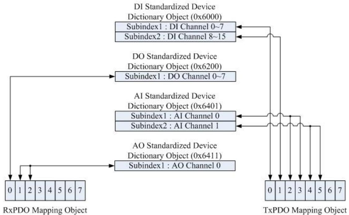
According to the PDO mapping objects in the figure above, if this CANopen device gets the RxPDO message including three bytes, the first byte is interpreted as the output value of the DO channels 0~7 and the following two bytes are the analog output value.
