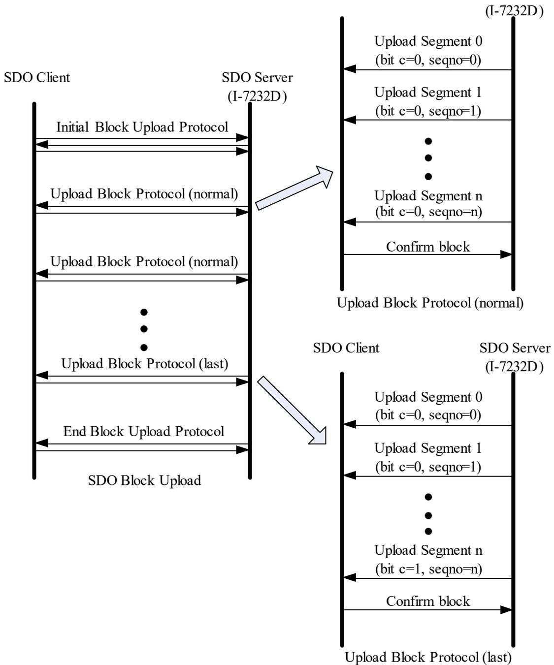
By following this procedure, we provide a demo for obtaining the value of the index 0x1008 and sub-index 00 object entries.
