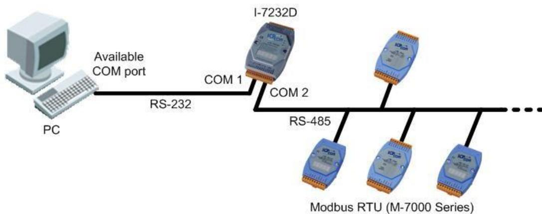
Step 1: First turn off the I-7232D. Connect the INIT\* pin and GND pin on the I-7232D. Then, turn on the I-7232D.
