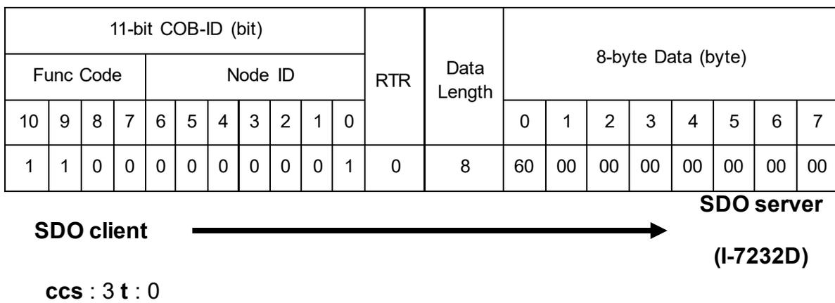
Step 4. I-7232D will respond to the first 8 bytes in the index 0x1008 and sub-index 00 object entries.
