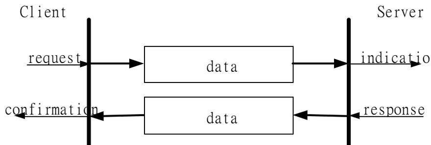
The SDO has two kinds of the COB-IDs, RxSDOs and TxSDOs. For example, from the view of the I-7232D, if users want to send a SDO message, then the I-7232D needs to receive the SDO message transmitted from users. Hence, the receive SDO (RxSDO) COB-ID of the I-7232D will be used.
