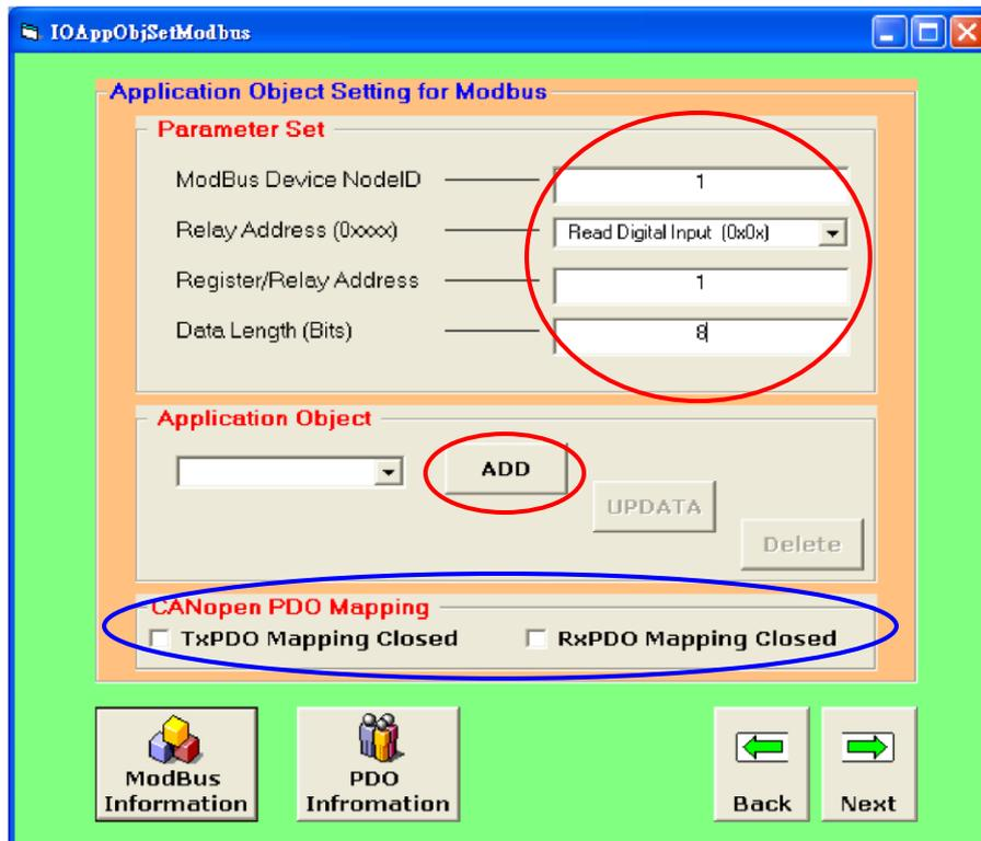
Users can click on the “PDO Information” or “Modbus Information” button to view the PDO objects or Modbus RTU devices configuration information. These information dialogs are shown below.
