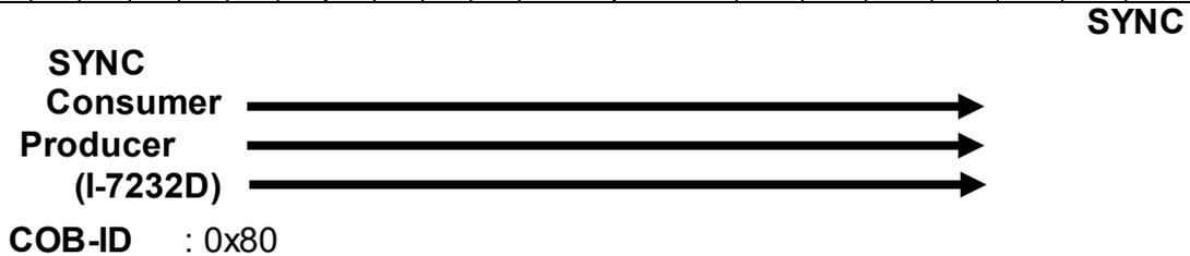
Step 26: After finishing the transmission of the three SYNC objects, the 1st TxPDO is triggered, and users can receive the 1st TxPDO from I-7232D.
