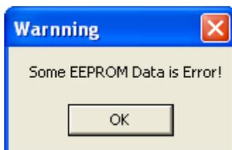
The default connected modules are I-7012, I-7021, I-7053 and I-7057. So if users connect the I-7231D with any different I/O module from the ones described above, then the "Some EEPROM Data is Error!" warning message may pop up. In this case, the default value will be shown on each parameter setting field. Otherwise, the last setting value will be displayed on each parameter setting field.
