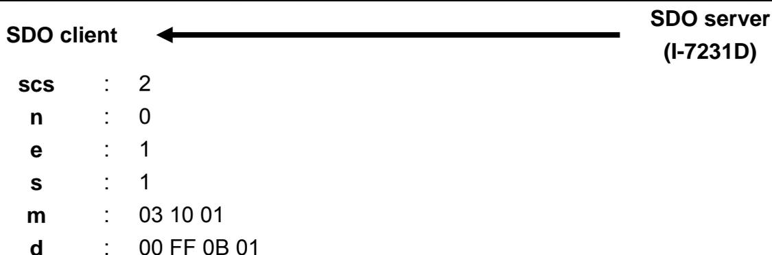
Step 5. Check the object 0x1001, and make sure that the manufacturer specific and generic errors on the error register are indicated.
