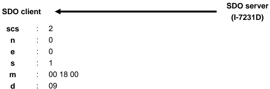
Because the first byte from the 8-byte data indicates that only the 4th byte is valid. Therefore, the feedback value is 09, and it means that there are 9 bytes to be uploaded.
