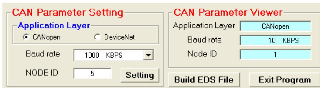
Step 6: Click the “COM2
