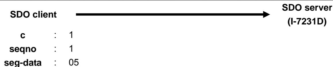
Step 4. The I-7231D responds to the message to confirm if the transmission is successful or not. If not, this block needs to be transmitted again. After finishing the data transmission, the Download SDO Block Segment protocol is terminated.
