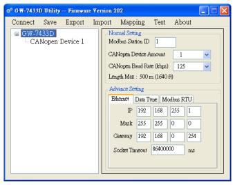
**Step4:** Because there are 4 CANopen slaves in this demo, select the "CANopen Device Amount" combo box to 4. And the device list in the left hand side will show 4 CANopen device items. If users want to change Modbus station ID and IP address, just input them in the suitable text box.
