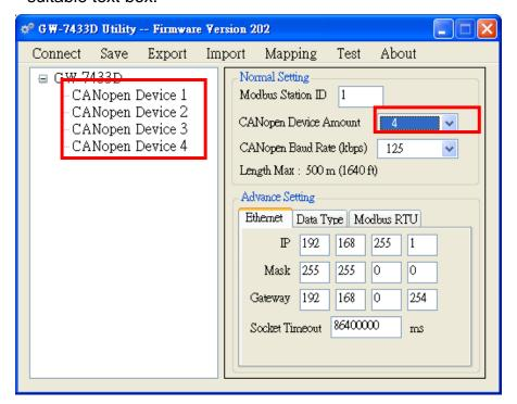
**Step5:** Click the "CANopen Device 1" item to configure the slave CANopen messages as following figure (assume that the device 1 is a 16-ch DO module with node ID 1). For example, add an RxPDO message with Cob ID 0x201 and 2-bytes Boolean data into the configuration of the GW-7433D.
