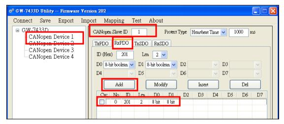
**Step6:** Click the "CANopen Device 2" item to configure the CANopen message as the following figure (the device 2 is a 16-ch DI module with node ID 2). This configuration is similar with the step 5. For example, add a TxPDO message with Cob ID 0x182 and 2-bytes Boolean data into the configuration of the GW-7433D.
