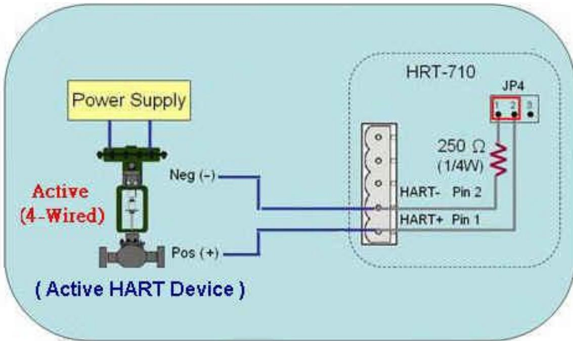
圖 13-3 : HART\_P2P\_Network\_Active (Built-In-Resistor)
