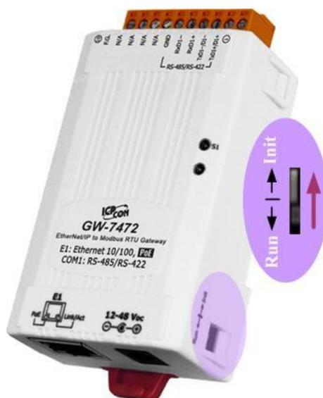
4. Connect both the GW-7472 and your computer to the same sub network or the same Ethernet switch, and power the GW-7472 on.
