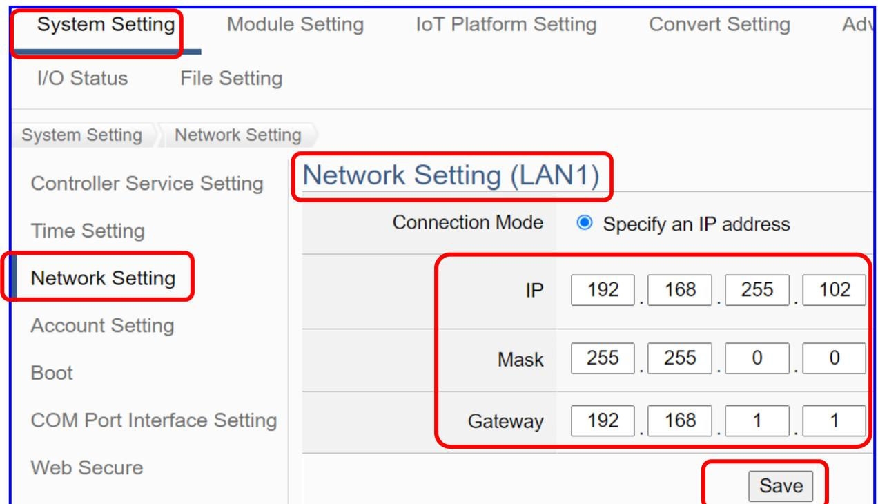
6. Save the IP setting, restore the PC original IP settings, and type the UA new IP in the browser to login the Web UI of UA-2200. And then configure user's UA project.
