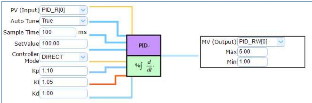
In the PID Operation function, UA controller collects the module’s data to operate via the feedback loop component of PID control. The controller compares the collected data with a reference value and then uses this difference to calculate a new input value whose purpose is to allow the system data to reach or remain at the reference value.
