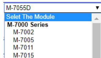
a) **Select The Module:** Select an ICP DAS model (as the pic), system will auto setup.
