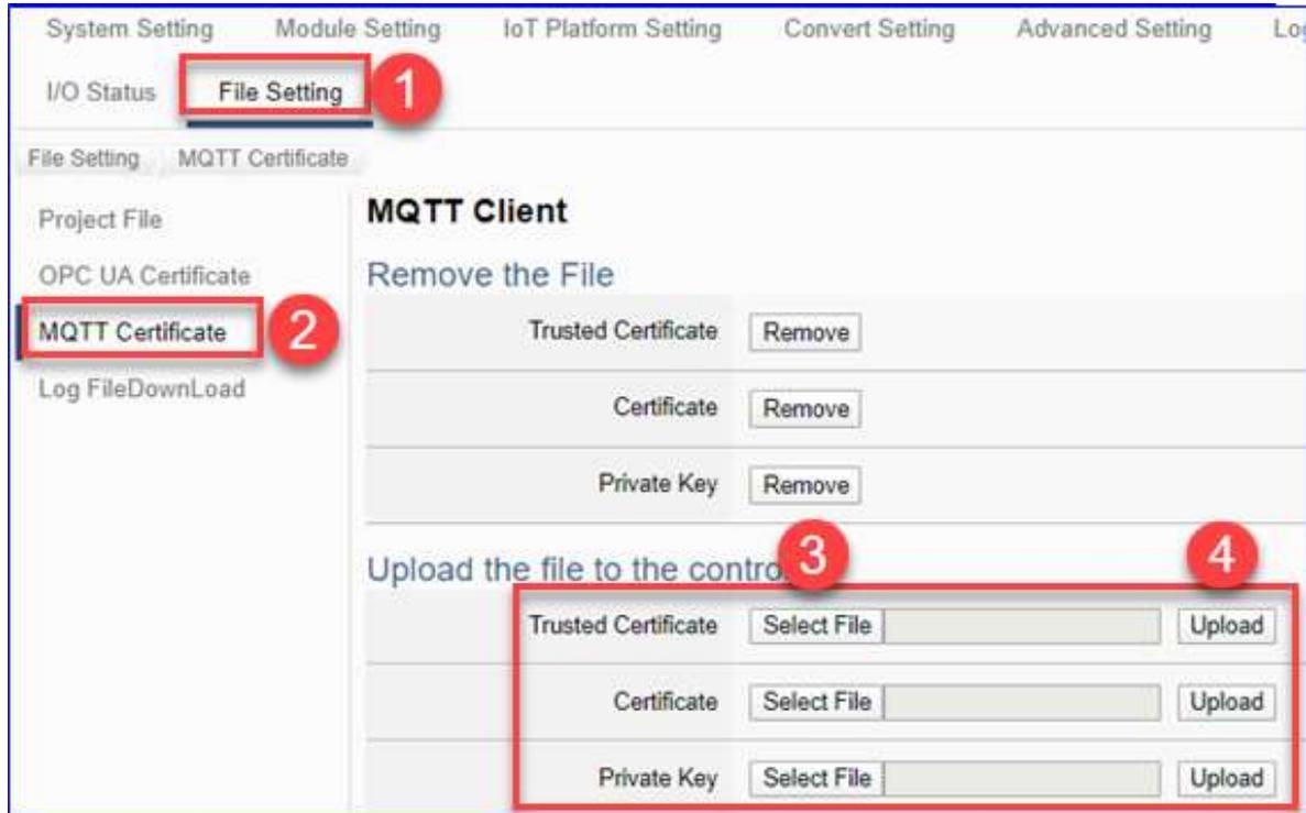
1. Get the trusted certificates from MQTT Client and save in the PC.
