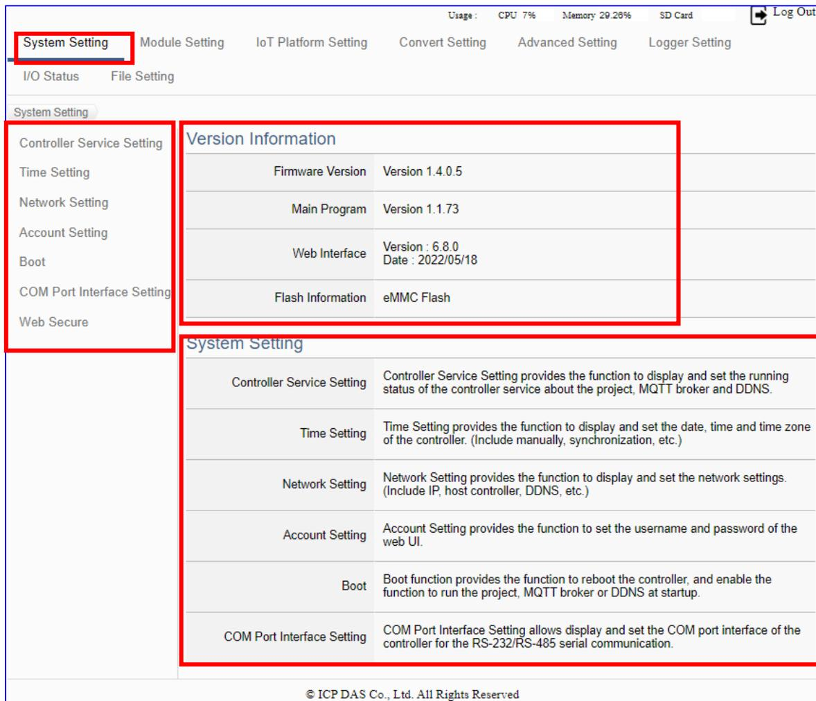
The setting for UA series controllers is to set up from the left to the right of the main menu functions. User can find the setting step and Web UI information in the following chapters.
