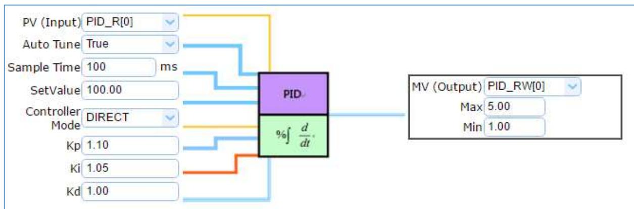
This section introduces the setting steps and the function parameters of the PID. There are 2 items about “PID” function in the “Function Wizard”. The 2<sup>nd</sup> item [PID Operation + OPC UA Communication Conversion] is combining the 1<sup>st</sup> item [PID Operation] and the FAQ. **The PID operation is for AI/AO data only, please select the AIO module when use the PID related Function Wizard.**
