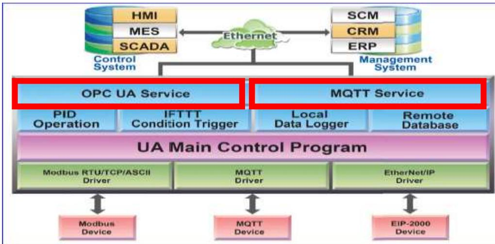
[IoT Platform Setting] includes five sub-menu functions in MQTT and OPC UA two connections and the function descriptions are listed on the page of the Main Menu, such as the Local Broker, Remote Broker, MQTT Group Connection and Microsoft Azure Platform in the MQTT Connection category, and the Local Server in the OPC UA Connection category. This chapter will introduce these function items and setting parameters.
