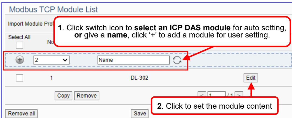
The function items and setting parameters of the [Modbus TCP Module List]:
