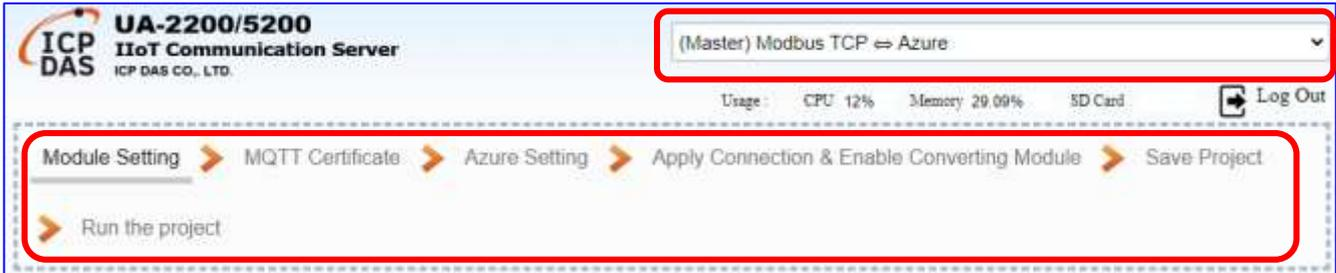
Step Box is a step guide of the Function Wizard. When users select an item, the Web UI will enable a Wizard and show a “Step Box” for user to follow the “Step Box” step-by-step and then can complete the project easily & quickly.
