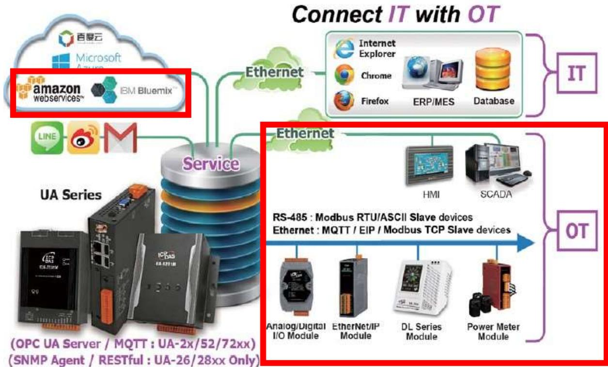
UA series controller built-in MQTT Broker, but when users want to use the external MQTT Broker, UA system also provides the settings to connect and publish/subscript messages with the MQTT Remote Broker.
