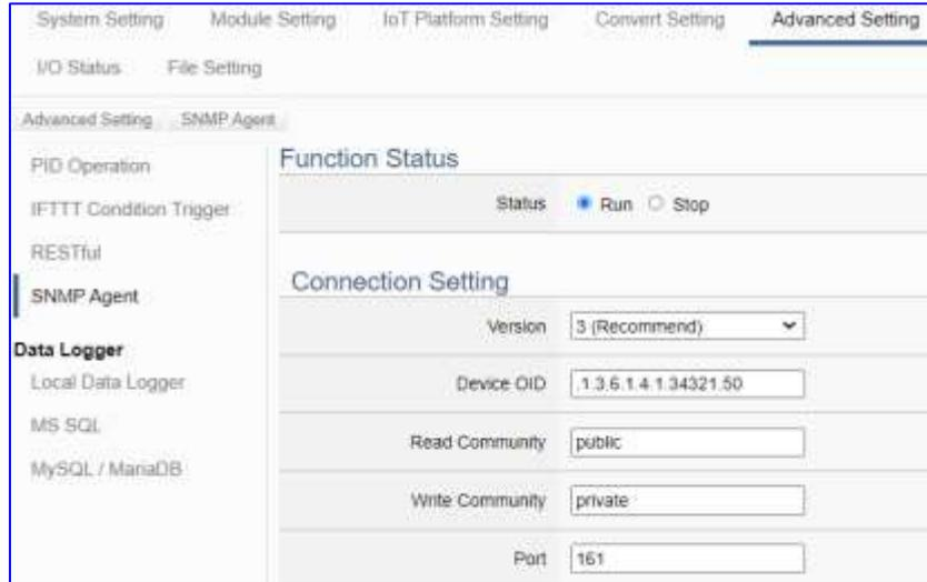
SNMP (Simple Network Management Protocol) is a communication protocol for managing network devices. It is one of the widely accepted communication protocols for managing and monitoring network elements. The user can use it in wireless networks to detect malicious wireless base stations. Network managers can isolate and dispose of them in real-time based on the detection results to avoid leakage of internal information or deliberate external attacks to maintain information security.
