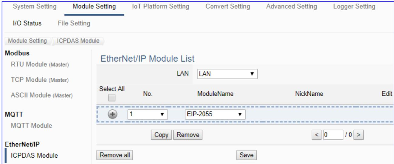
This page is for setting the communication values with the connected EIP modules. First, choose the Ethernet LAN port that connected with the module, and select the name of EIP module. Click [ + ] button could add a new module, and then click [Edit] button to configure the module content and the MQTT variable table.
