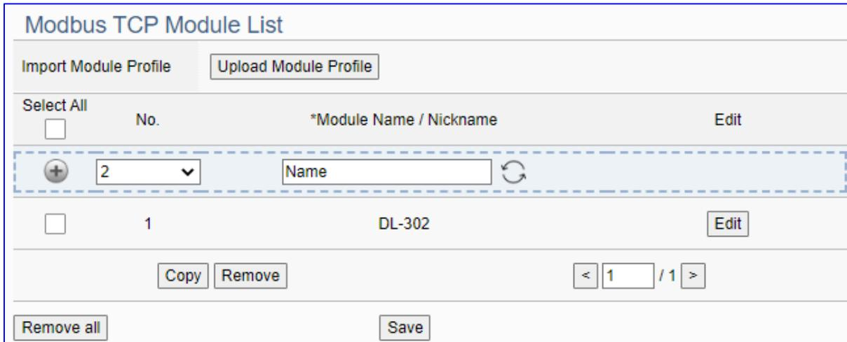
This section shows the settings for the Modbus TCP module on Ethernet LAN. User can give module a name (Default: Name), click [ + ] button to add a new module, and then setup the module. If using ICP DAS module, user can just select the model, system will auto add and setup the module. Click [Edit] button to set the module content and the Modbus mapping table.
