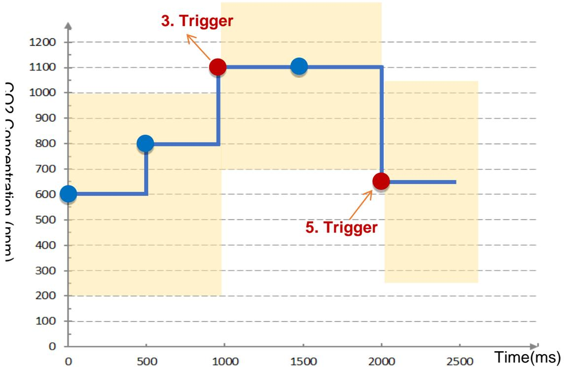
**AIO Trigger:** (Detect per 500 ms. The yellow block means the Dead Band.)
