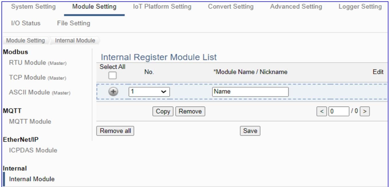
This page is for setting the internal module list. First, enter the name for the module. Click [ + ] button to add a new module, and then click [Edit] button to configure the module variables.
