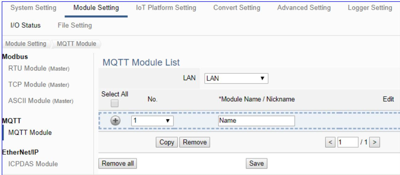
This page is for setting the communication values with the connected modules. First choose the Ethernet LAN port that connected with the module, and each module can give a name (Default name: Name). Click [ + ] button could add a new module, and then click [Edit] button to configure the module content and the MQTT variable table.
