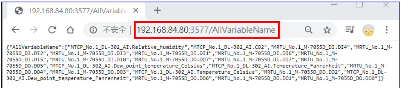
From the upper web browser and the lower UA web interface, the user can find that UA supports directly request all the I/O variable data of the connected modules DL-302 and M-7055D via the web browser.
