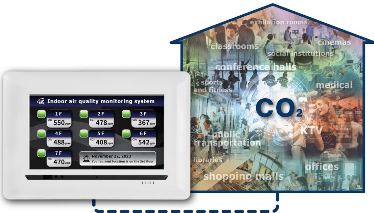
The ICP DAS TPD-703-64 has RS-232/RS-485 and Ethernet communication interfaces to collect data from central control systems or on-site air quality sensors. The 7" touch screen can display multiple pages to show more air quality information for the general public or for the site manager's reference for crowd control.
