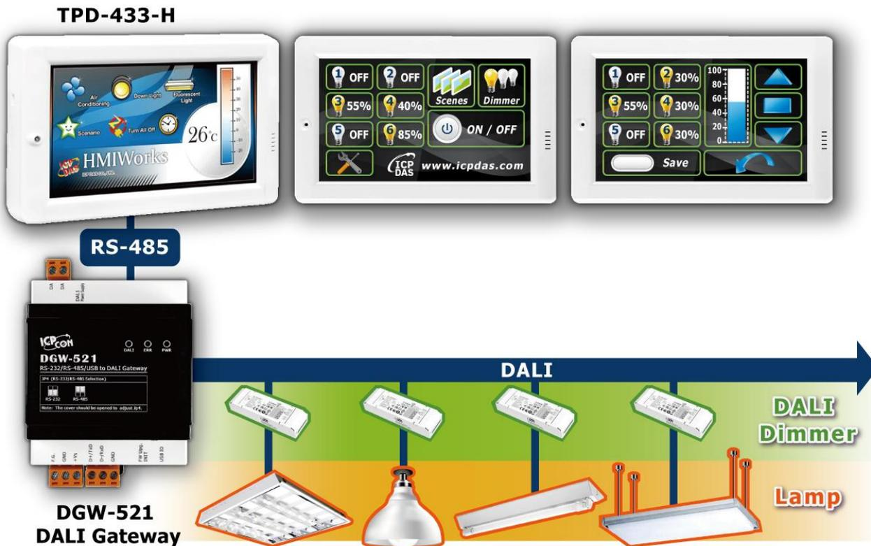
The traditional 0-10V analog signal dimming method has problems such as deviation or jump due to signal interference and voltage instability. Digital DALI can provide 255 levels of fine and stable dimming, which can be controlled individually, in groups or broadcast. With the support of custom scene mode, the lighting brightness of each area can be pre-configured and the scene can be switched with a single command.
