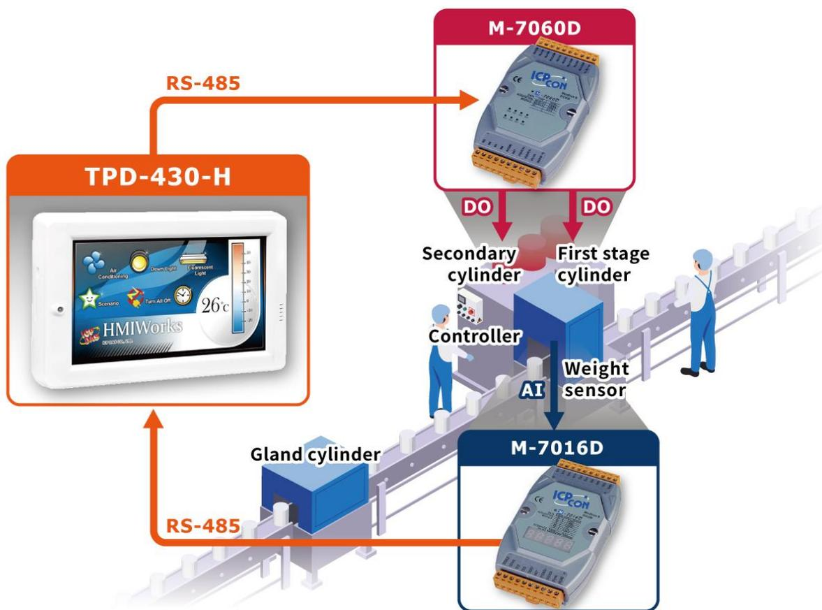
Using TPD-430-H as the main controller, the touch screen allows the operator to set the system parameters such as: empty and full drum weight value, primary and secondary cylinder off value...etc. The weight sensor output value is read by the M-7016D, and the TPD-430-H is used to filter the small jump value and determine the start/stop of the filling operation based on this weight data.
