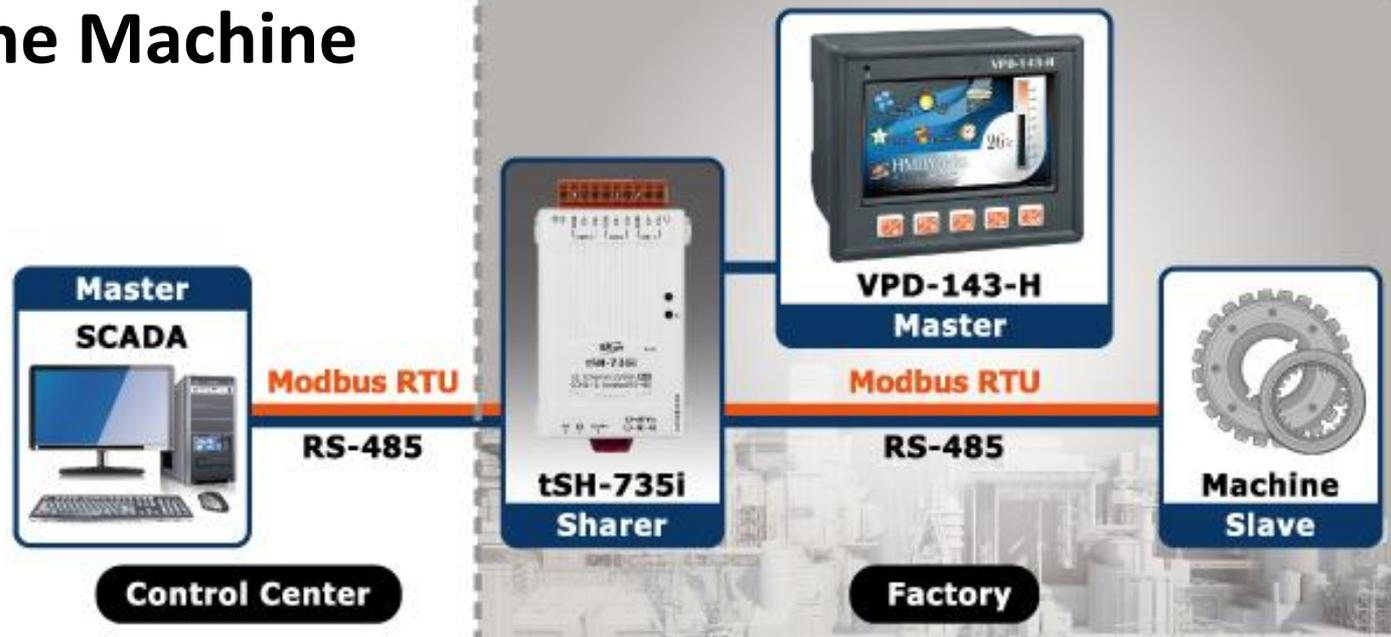
The original architecture is a remote SCADA (Supervisory Control and Data Acquisition) system connected to the machine at the factory via RS-485 for monitoring and setting. With the introduction of tSH-735i and VPD-143-H, the original remote SCADA system can still work with the machines, and the field personnel can also check and adjust the parameters of the machines in the factory to improve the efficiency of the field work.
