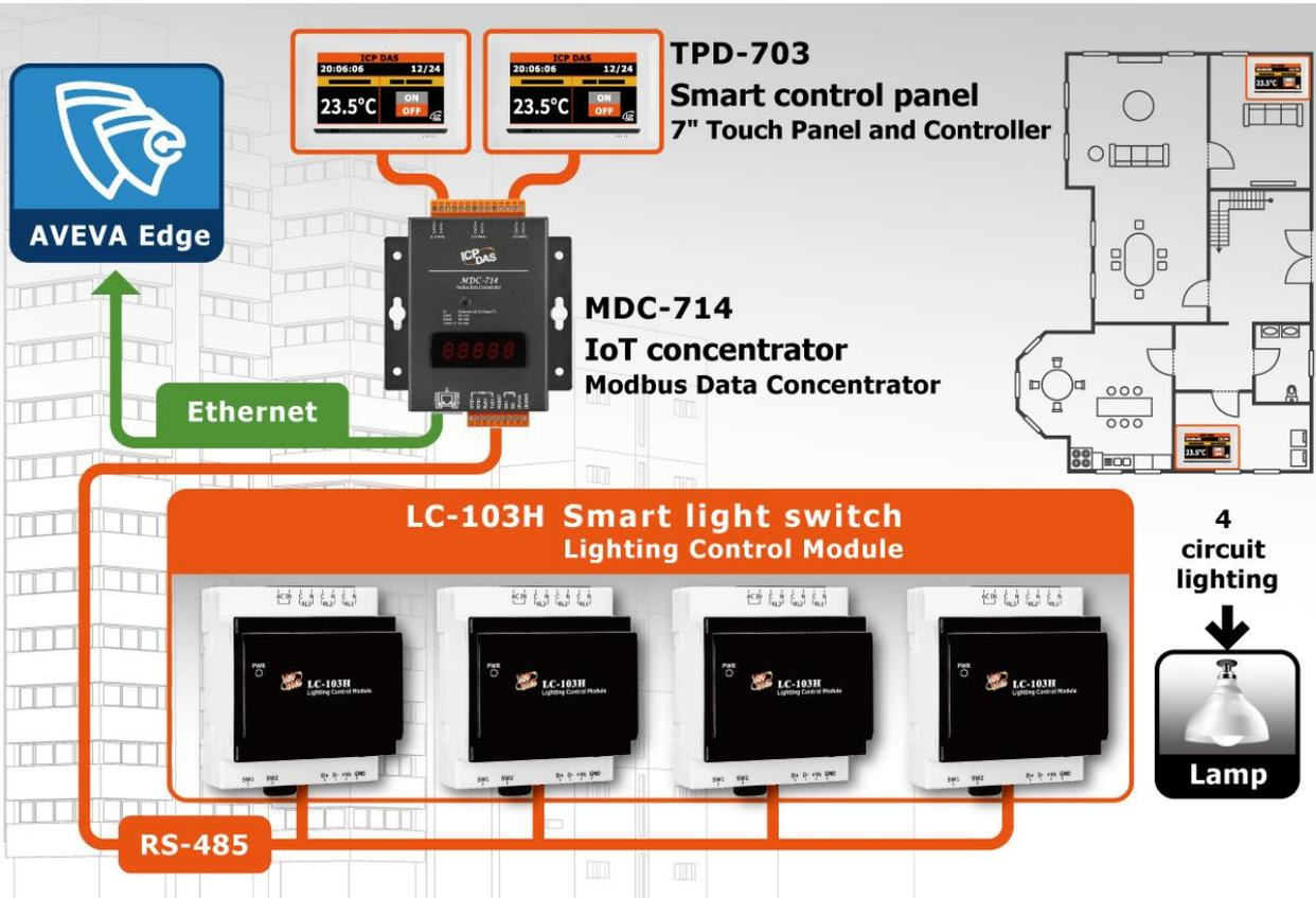
A building has several lighting systems, including office lights on each floor, public area lights, and LED lights on the exterior of the building. Previously, a timer was used in each area to turn the lights on at night and off during the day, but it was inconvenient and time-consuming for the maintenance staff to change the settings each season.
