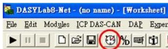
Step 6: Select the "Driver" and "ICP DAS-CAN" tab. Set the sample rate to 200Hz and block size to 1.
