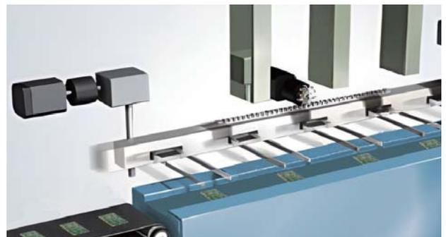
▲ Simultaneous activation of multi-axis motors
