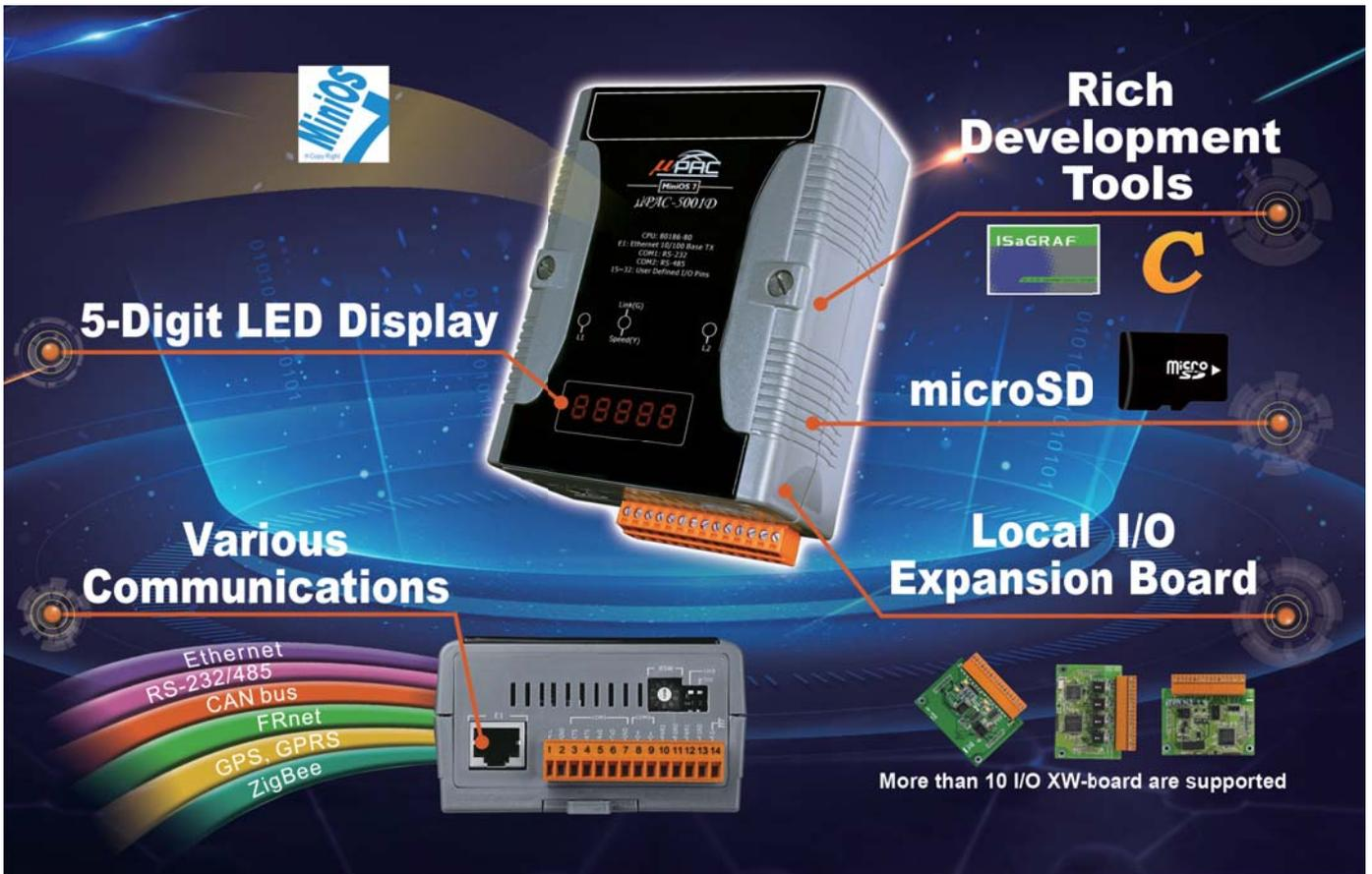
The uPAC-5000 Series is equipped a 80186 CPU running a MiniOS7 operating system, a variety of connectivity options (Ethernet, RS-232/485) and an I/O expansion bus.
