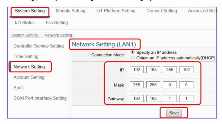
**6.** Save the IP setting, restore the PC original IP settings, and type the UA **new IP** in the browser to login the Web UI of UA-7200. And then configure user's UA project.
