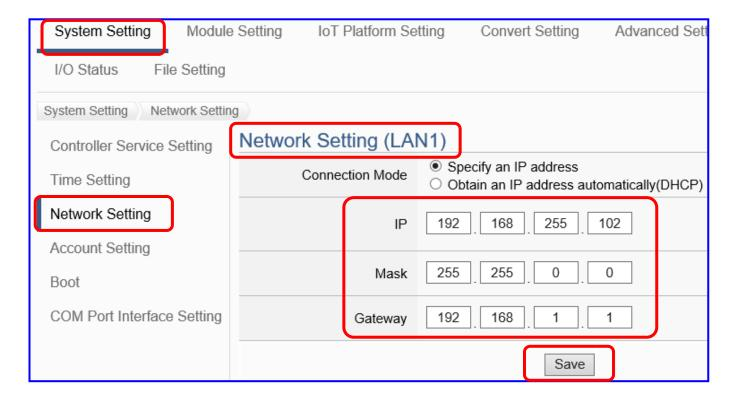
6. Save the IP setting, restore the PC original IP settings, and type the new IP in the browser as step-3 to login the Web UI of UA-2800. And then configure user's UA project.
