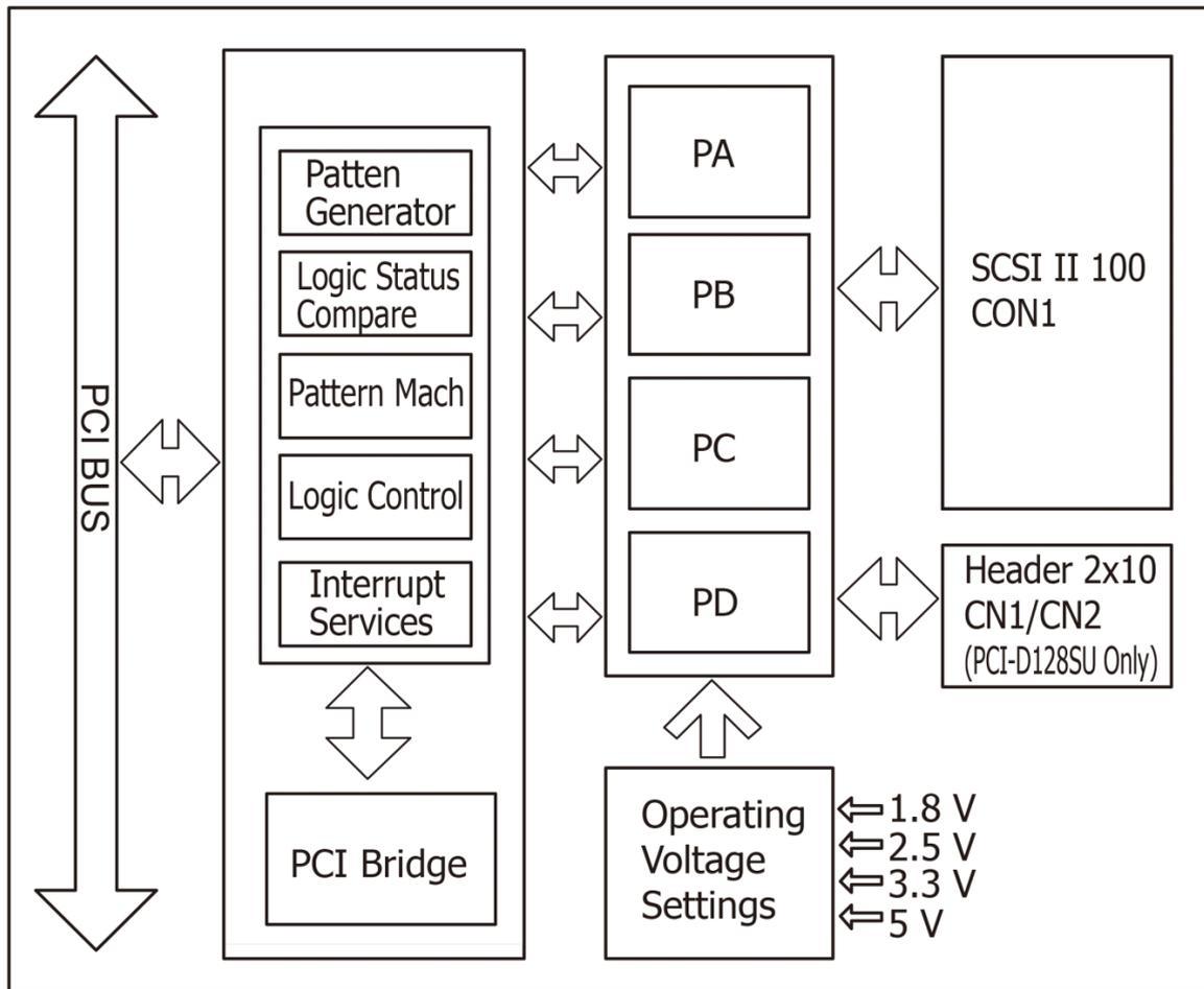
Figure 1-3: Block Diagram of PCI-D96SU/D128SU
