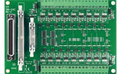
The transistor is energized by applying a 5-voltage signal to the appropriate input channels on the 50-pin header or 20-pin header or 37-pin D-sub connector. Twenty-four enunciator LEDs, one for each transistor, light when their associated transistor is activated. The DB-24C daughter board is connected to the CN1/CN2 connector on the D128SU using a 20-pin flat cable.
