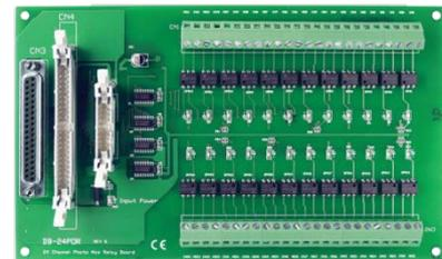
The relay is energized by applying a 5 voltage signal to the appropriate relay channel on the n the 50-pin header or 20-pin header or 37-pin D-sub connector. Twenty-four indicators LEDs, one for each relay, light when their associated relay is activated. The DB-24POR daughter board is connected to the CN1/CN2 connector on the D128SU using a 20-pin flat cable.
