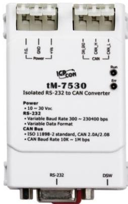
The left graph is the surface of tM-7530. It uses D-sub 9 pin female connector as RS-232 communication interface and uses 2 or 3 wire to connect CAN bus with spring type connector. It has 2 LED indicators Run and Err. They are used to response module status immediately at all time.
