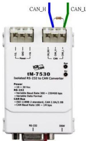
There is no terminator resistor in the tM-7530. Therefore, if users would like to use terminator resistor, it is necessary to wire a 120Ω resistance on the CAN bus, as following figure.
