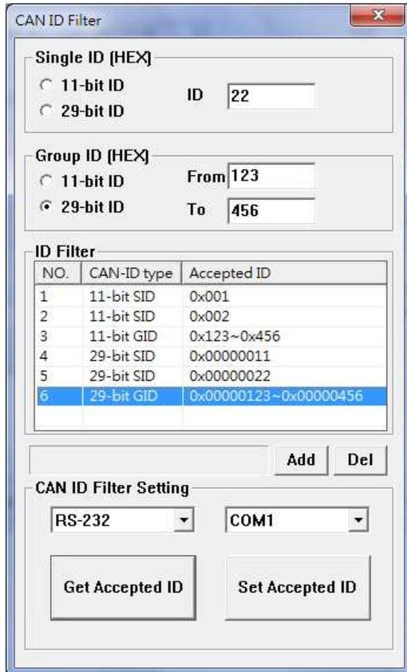
Figure 3-11: CAN ID Filter Settings Screen
