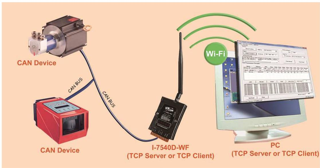
Figure 4-2: I-7540D-WF application architecture (I-7540D-WF + PC)
