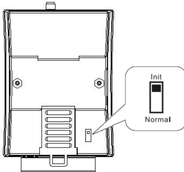
Figure 2-10: Init Position of Dip-Switch
