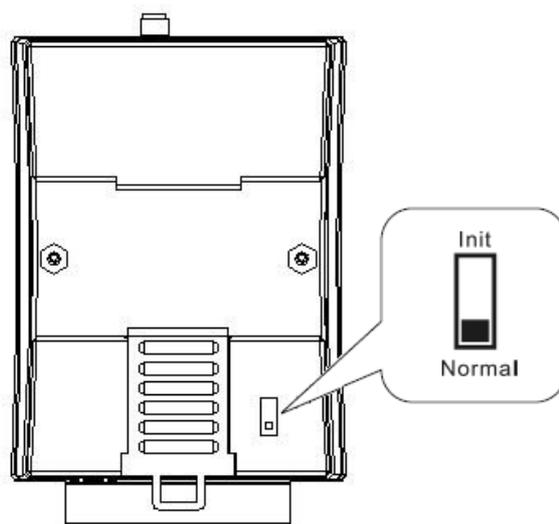
Figure 2-14: Normal Position of Dip-Switch
