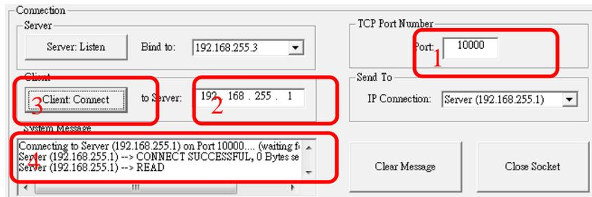
Figure 4-11: I-7540D-WFUtility-Client connection procedure
