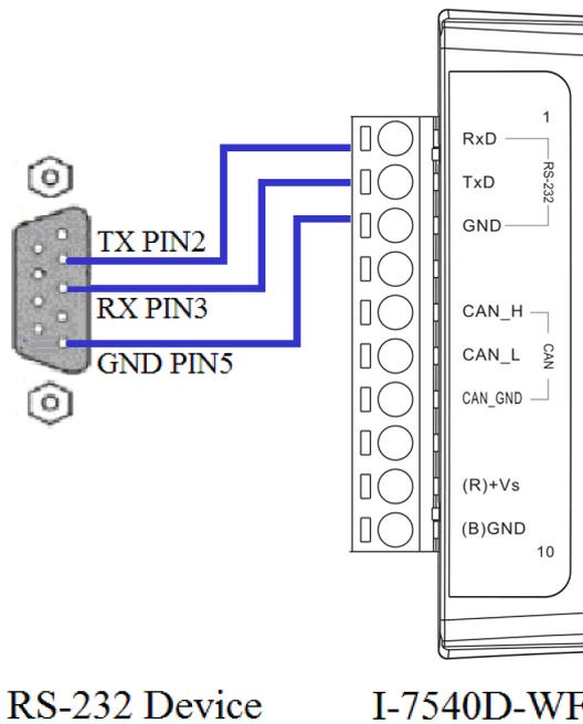
Figure 2-5: RS-232 Wire Connection
