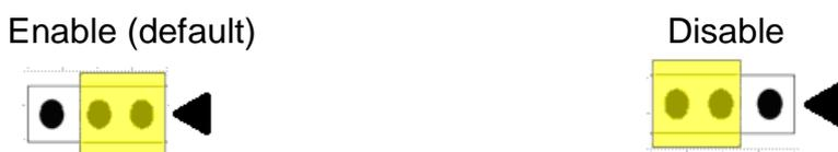
Figure 2-8: Terminal resistor JP2 Jumper Position
