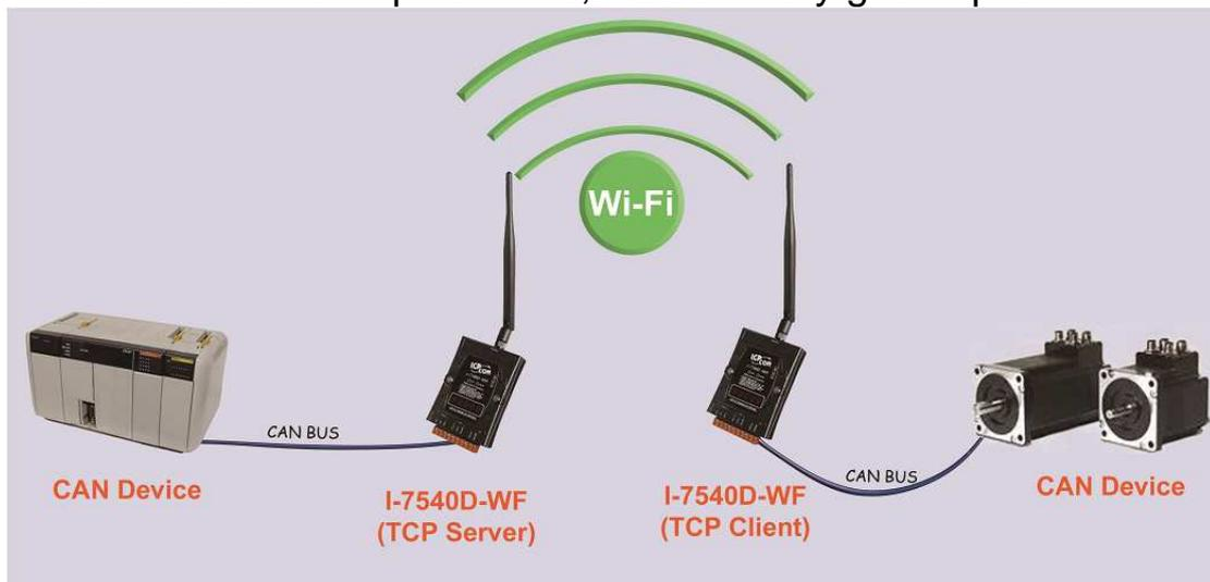
Figure 4-1: I-7540D-WF application architecture (two I-7540D-WF)
