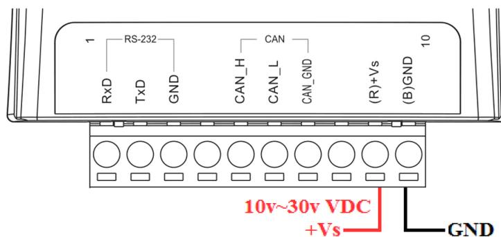
Figure 4-3: Power Wiring
