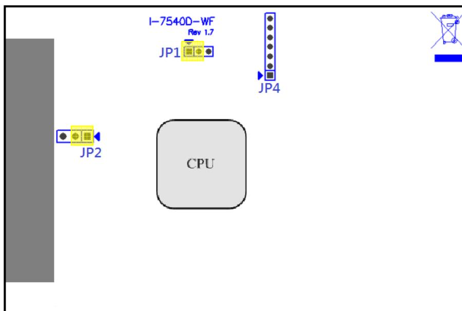
Figure 2-7: Terminal Resistor Jumper
