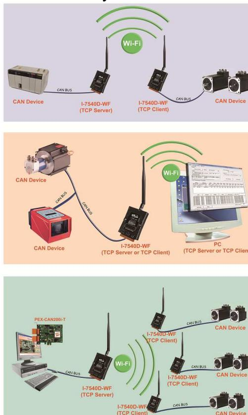
Figure 1-1: Application architecture for the I-7540D-WF
