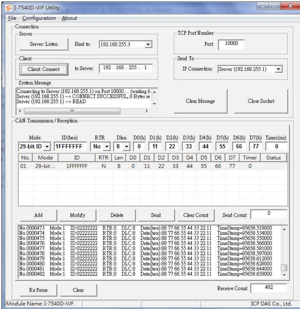
Figure 3-12: I-7540D-WF Utility Main Screen
