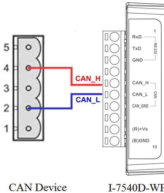
Figure 2-4: CAN Hardware Wire Connection
