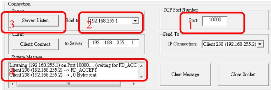
Figure 4-12: I-7540D-WFUtility-Server connection procedure
