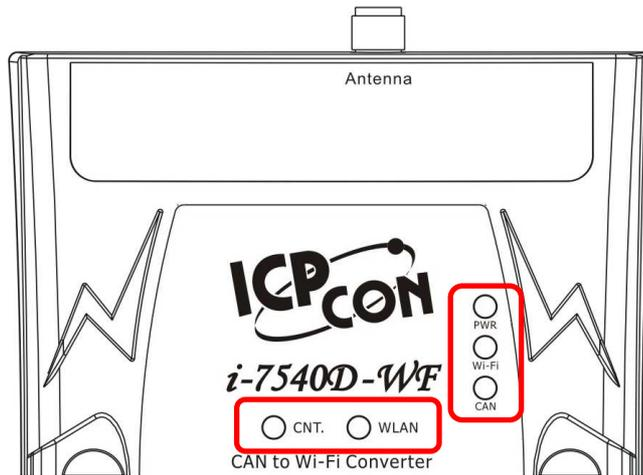
Figure 2-15: LED position of the I-7540D-WF
