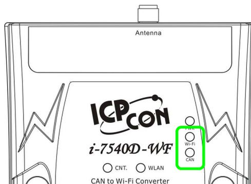
Figure 4-10: I-7540D-WF CAN and Wi-Fi Transmission LED
