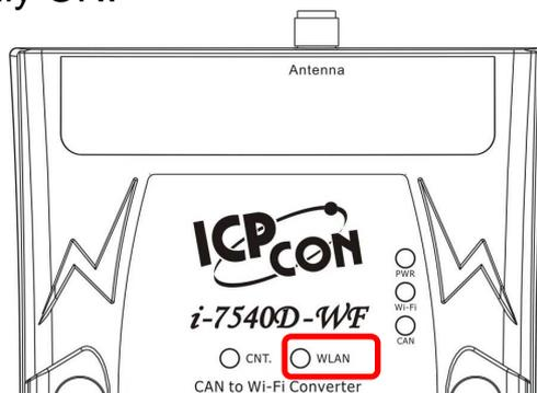
Figure 4-7: Ad-Hoc connection LED
