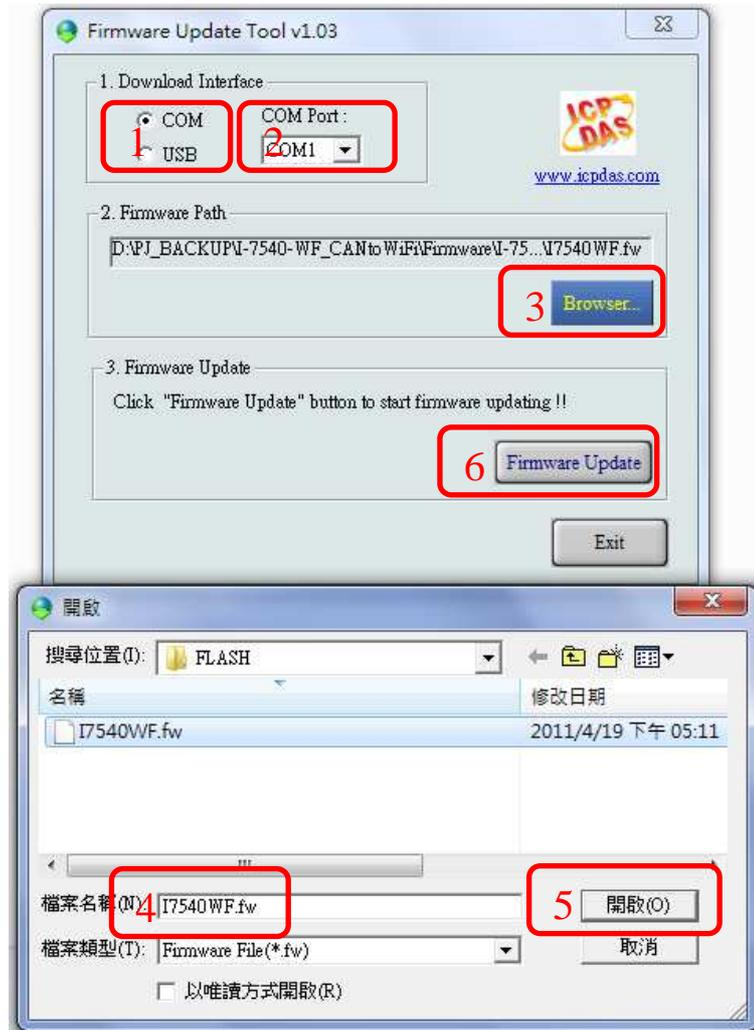
Figure 2-13: I-7540D-WF firmware update process
