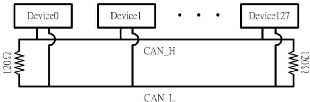
Figure 2-6: Terminal Resistor
