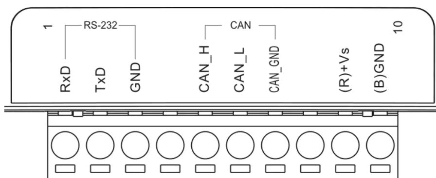
Figure 2-3: Pin Assignment on the I-7540D-WF
