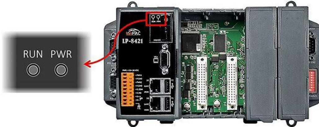
Figure 6.5.3-1. LED indicators for LP-8x2x series
