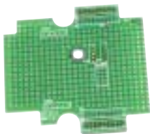
Self-test Board X003 (64mm x 32mm)
