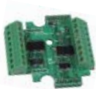
D/I/O Board **Without Case** X119 (72mm x 57mm)
