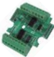
DI/O Board X119 (72mm x 65mm); 0.5W
