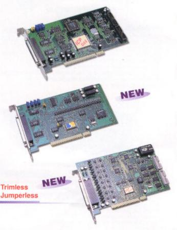
PCI-1002: Cost-effective multi-channel A/D board,12-bit resolution, 125K sampling rate, 32single-ended/ 16 differential channels, 16-channel D/I, 16-channel D/O
